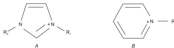
Fig. 1. Generic structure of 1-alkyl-3-methylimidazolium (A) and N-methylpyridinium (B) ionic liquid cations. R 1 , methyl – decyl; R 2 , methyl – etyl.
