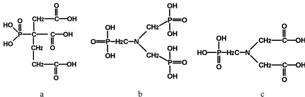
Fig. 1. Structural formulas of 2-phosphonobutane-1,2,4-tricarboxylic acid – PBTC (a), N-trismethylenephosphonic acid – NTMP (b) and N-(phosphonomethyl)iminodiacetic acid – PMIDA (c).
