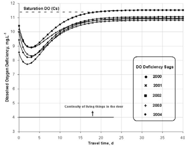
Fig. 4. Variation of DO profile according to time for the Stream (the annual average values).
