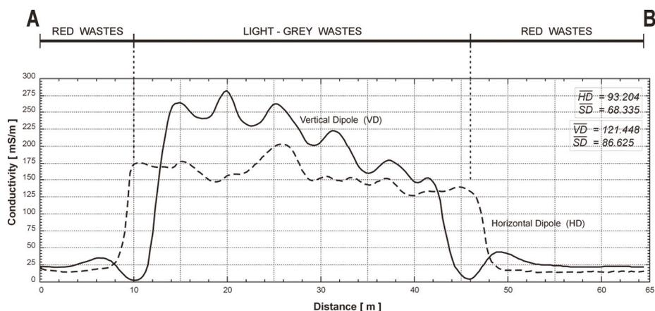
Fig. 5. Variations of apparent electrical conductivity along A-B reference profile to a depth of approx. 3 m (HD) and approx. 6 m (VD). (EM31-MK2 conductivity meter).
