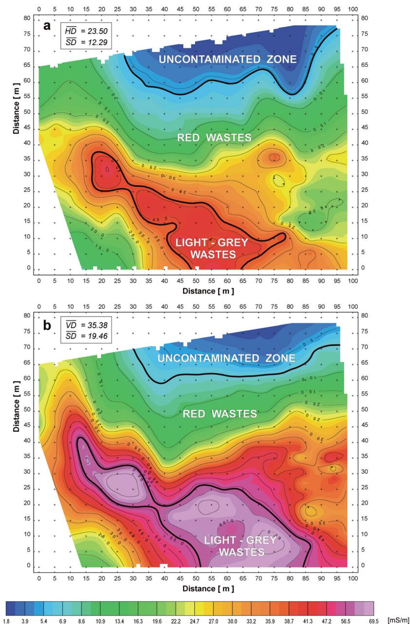
Fig. 4. Maps of apparent electrical conductivity to a depth of:
