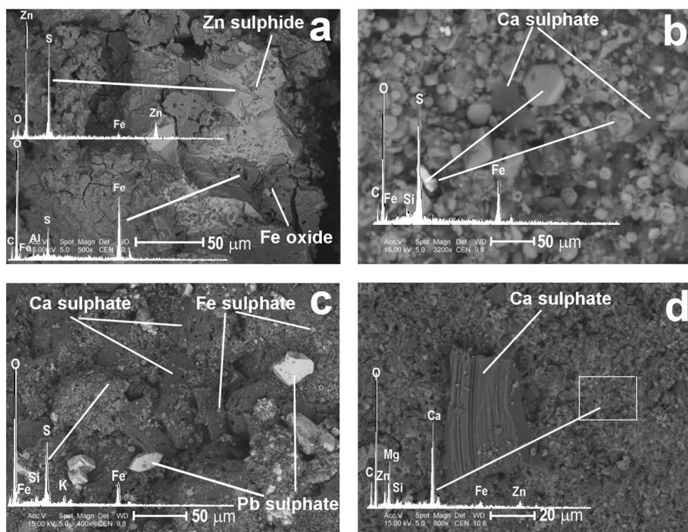
Fig. 3. BSE images of metal-bearing components in the waste from historical Zn-Pb ore processing.
