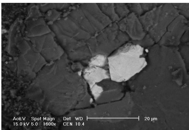
Fig. 4. Barite particles (white points) in ash from domestic furnace.
