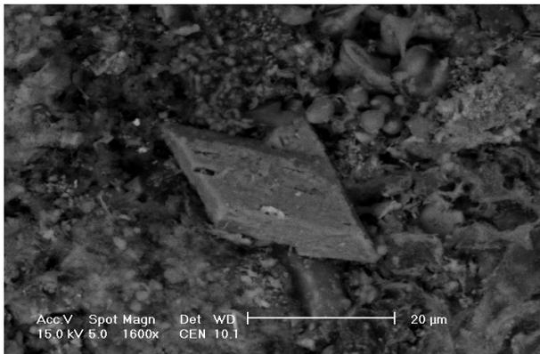
Fig. 3. Gypsum twin in ash from domestic furnace.
