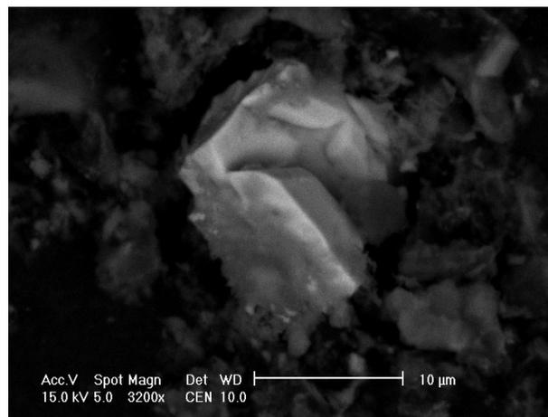
Fig. 7. SEM image of monazite particle in ash from domestic furnace.
