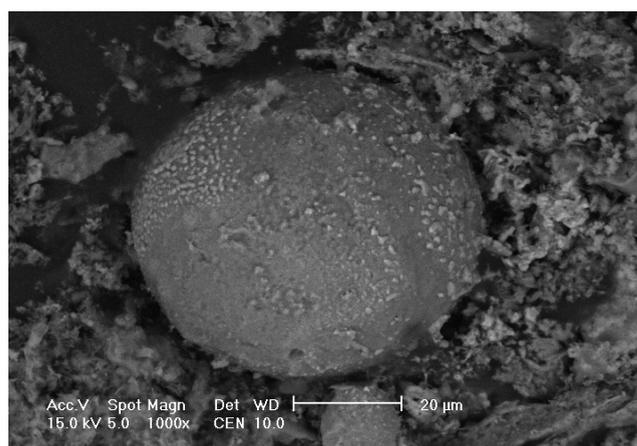
Fig. 1. SEM image with EDS spectrum of aluminosilicate particle in ash from domestic furnace.
