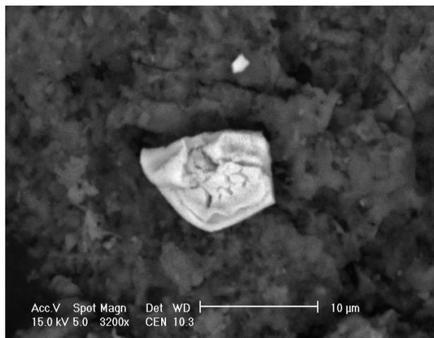
Fig. 2. SEM image with EDS spectrum of PbS in ash from individual domestic furnace.
