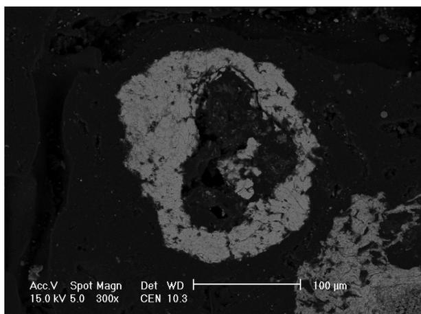
Fig. 6. SEM image of iron oxides particles in ash from domestic furnace.
