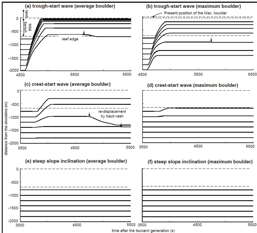
Fig. 5. Time series variation of the positions of (a) average and (b) maximum boulders by the trough-start wave, (c) average and (d) maximum boulders by the crest-start wave, and (e) average and (f) maximum boulders by the trough-start wave with a slope inclination of 1/10. Arrows indicate the onset of the movement of boulders seaward by backwash.
