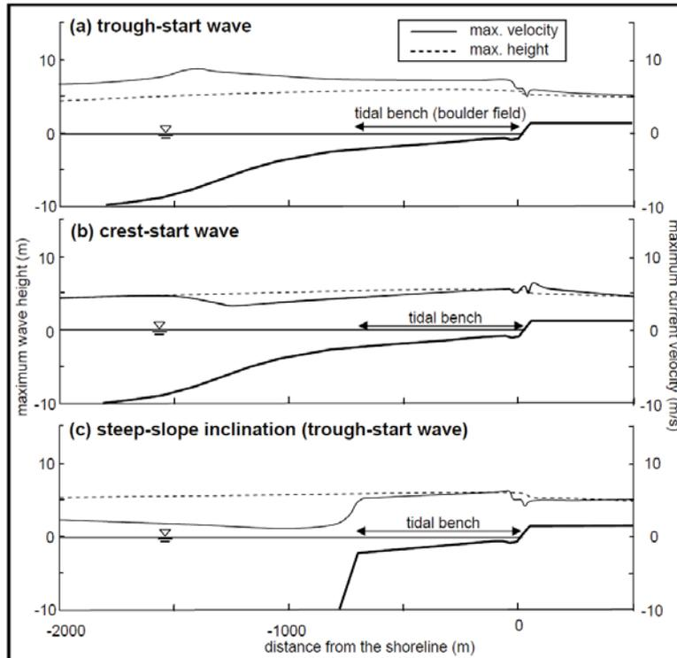
Fig. 4. Numerical results of the maximum current velocity (solid line) and wave height (dotted line) during the calculation time for (1) a trough-start wave, (2) a crest-start wave, (3) and a trough-start wave with slope inclination of 1/10.
