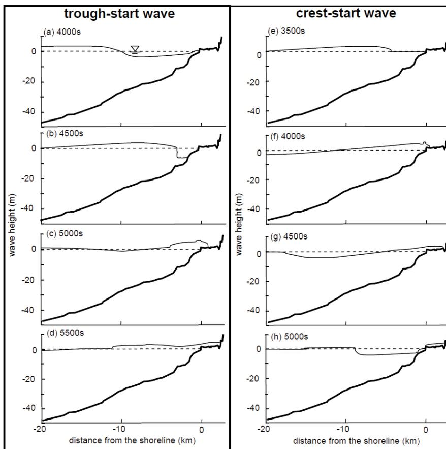
Fig. 3. (a)-(d) Snapshots of computing inundation pattern of the trough-start wave at 4000-5500 s after tsunami generation, and (e)-(h) of the crest-start wave at 3500-5000 s after the tsunami generation. Dotted and solid lines respectively mark the still water depth and tsunami wave.
