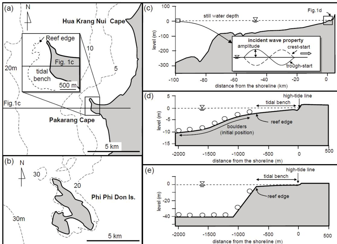
Fig. 1. (a) Location map of the studied area at Pakarang Cape, Thailand. (b) Bathymetry around Phi Phi Don Island, Thailand. Its difference from the bathymetry from that of Pakarang Cape is noteworthy. (c) Schematic diagram of the coastal profile and incident wave used for this study. (d) Schematic diagram of the coastal profile near Pakarang Cape. Original positions of boulders are also shown. (e) Schematic diagram of the coastal profile that was modified to be a reef slope inclination of 1/10.
