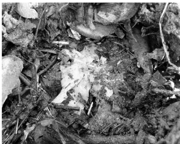
Fig. 2. The compost in which the samples studied were embedded (foil composed of starch, glycerine and montmorillonite after 23 days of biodegradation).
