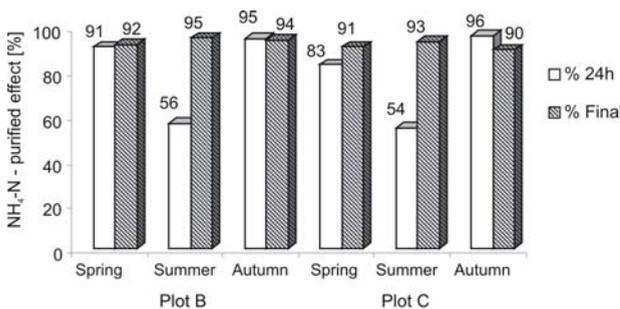
Fig. 4. Effect of wastewaters purification for ammonium ion (%) during the first day and at the end of the experiment.
