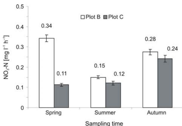
Fig. 6. Reduction of NO<sub>3</sub><sup>-</sup>-N (mgL<sup>-1</sup>h<sup>-1</sup>) in drainage waters with relation to irrigation dose and season of the year for the first 24 hours of the experiment.
