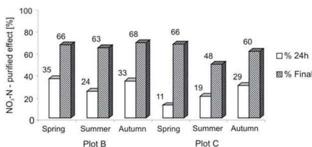
Fig. 7. Effect of wastewater purification for nitrate(V) ion (%) during the first day and at the end of the experiment.
