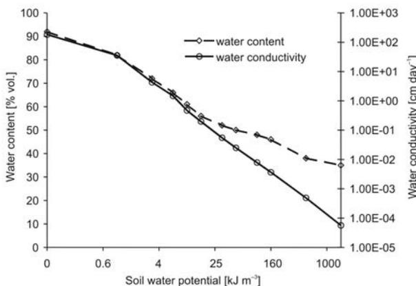
Fig. 1. Water content and water conductivity at different soil water potential.
