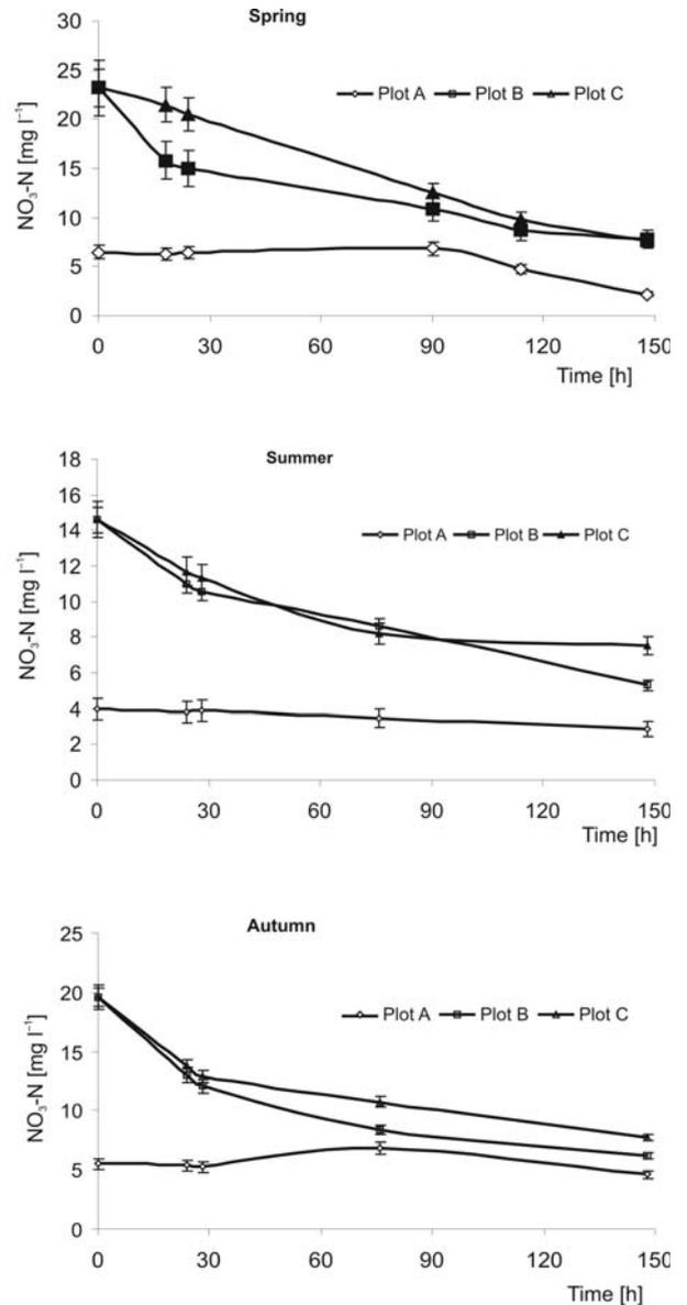
Fig. 5. Concentration of NO<sub>3</sub><sup>-</sup>-N (mgL<sup>-1</sup>) in drainage waters as a function of time and irrigation dose.
