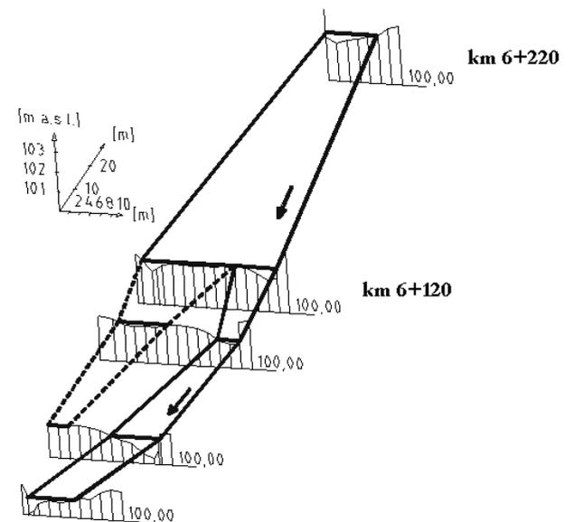
Fig. 3. 3D view of the research reach of the Mszanka Stream, October 1996. The solid line represents the water surface level borders in the main stream. The broken line represents the water surface level for the secondary stream.
