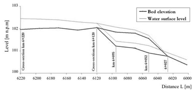
Fig. 2. The longitudinal profile of the research reach of the Mszanka Stream, October 1996.
