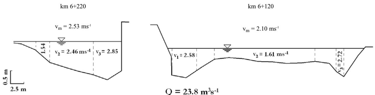
Fig. 6. Water flow velocity along cross-section for discharge  $Q = 23.8 \text{ m}^3 \cdot \text{s}^{-1}$ , Mszanka Stream. The broken lines define subsections of the cross-section division for which local velocities, shear stresses and stream power were calculated.
