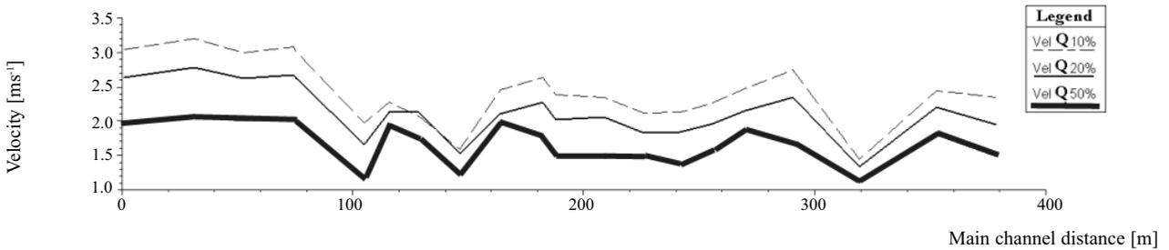
Fig. 7. Total water flow velocity  $v_m$  along the research reach for discharge  $Q_{50\%}$ ,  $Q_{20\%}$ , and  $Q_{10\%}$ , Targaniczanka Stream, 2004.
