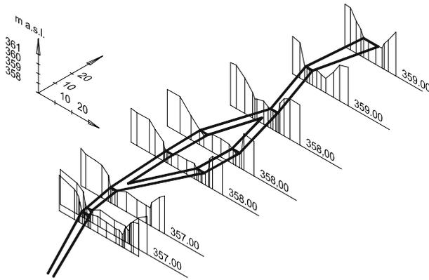
Fig. 5. 3D view of upper part of the research reach of Targaniczanka Stream, 2006.
