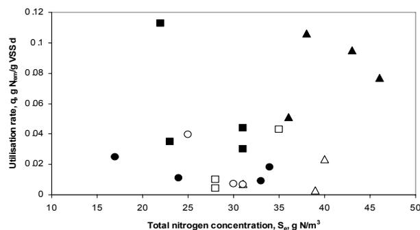
Fig. 5. Total nitrogen utilization rates versus its concentration in the final effluent (solid symbols – CFR, empty symbols – SBR) (circles – R1, squares – R2, triangles – R3).
