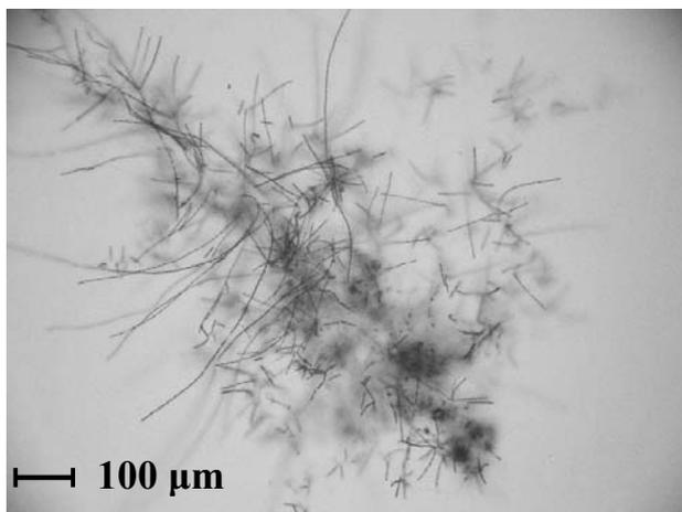
Fig. 8. Dominating filamentous organisms in reactor R2 during stage II.
