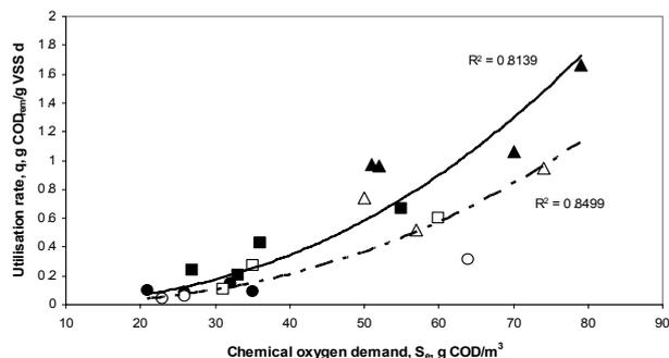
Fig. 2. Organic carbon utilization rates as functions of COD in the final effluent (solid symbols and line – CFR, empty symbols and dashed line – SBR; circles – R1, squares – R2, triangles – R3).
