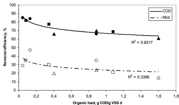
Fig. 4. Organic carbon and total nitrogen removal efficiency in SBRs as a function of organic load (circles – R1, squares – R2, triangles – R3).
