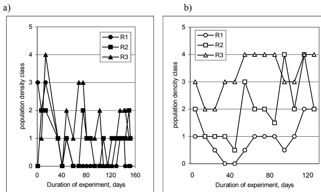
Fig. 7. Number of filamentous microorganisms in the activated sludge: a) CFRs, b) SBRs
