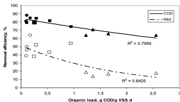
Fig. 3. Organic carbon and total nitrogen removal efficiencies in CFRs as functions of organic load (circles – R1, squares – R2, triangles – R3).
