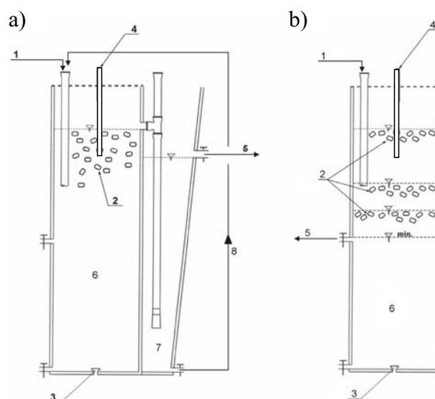
Fig. 1. Experimental set-up. a) CFR, b) SBR; 1 – inlet of septic tank effluent, 2 – moving carriers, 3 – air diffuser, 4 – oxygen measurement port, 5 – outlet of treated sewage, 6 – reactor, 7 – secondary clarifier, 8 – recirculation.
