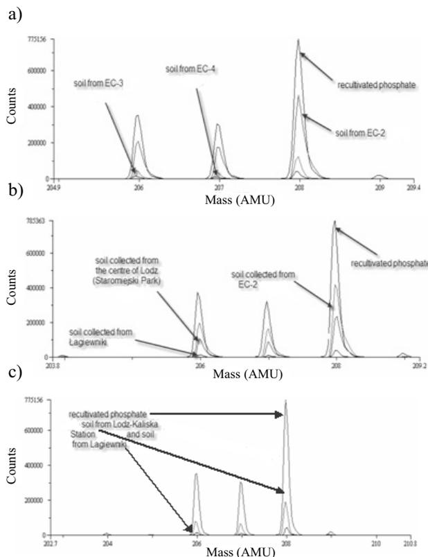
Fig. 7. The differences in the number of counts for lead isotopes (<sup>206</sup>Pb, <sup>207</sup>Pb, <sup>208</sup>Pb) for samples collected from the recultivated part of phosphogypsum and chosen sampling sites in Łódź (a, b, c). Generally, the lowest number of counts for lead is recorded for control – Lagiewniki Forest and the highest for recultivated phosphate.
