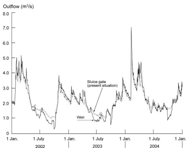
Fig. 8. Changes in outflows from Žuvintas Lake after replacing the sluice-gates (present situation) with a weir.
