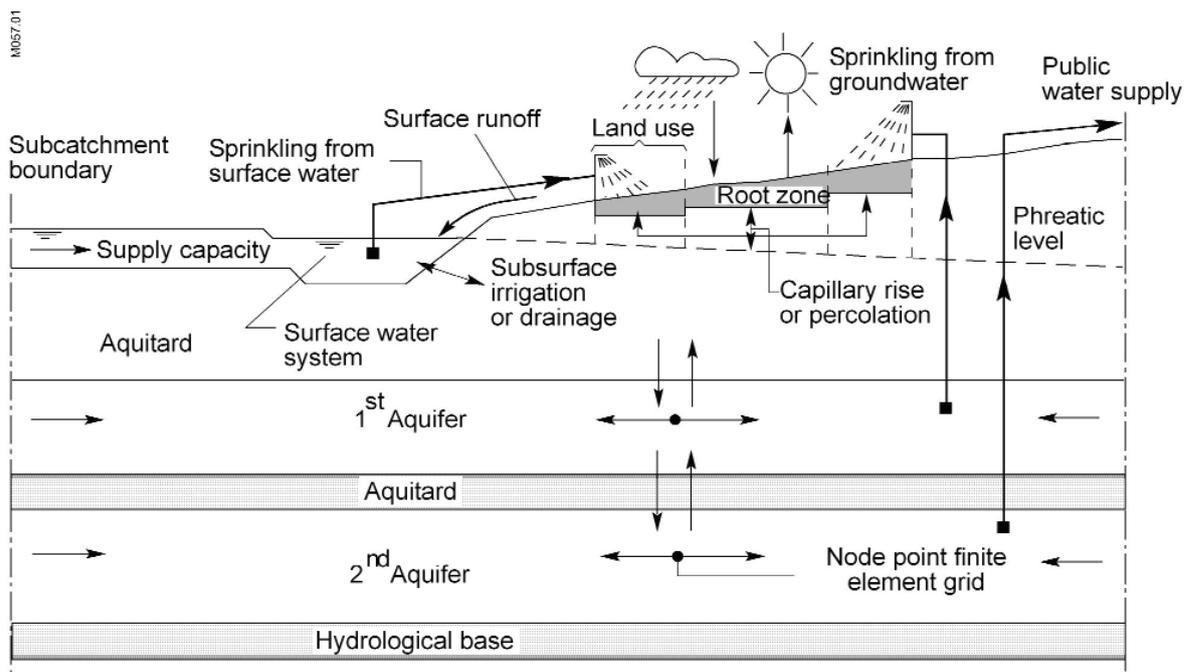
Fig. 1. Schematization of water flows in the SIMGRO model. The main feature of this model is the integration of a saturated zone, unsaturated zone and the surface water systems within a subcatchment [14].
