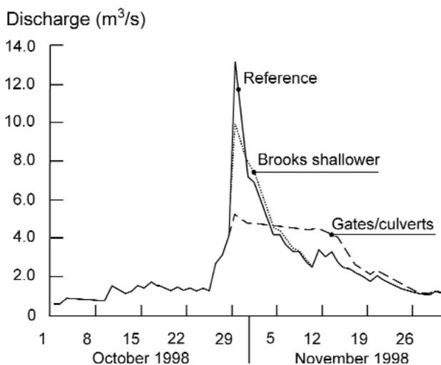
Fig. 3. Discharges for reference situation and the two measures for an extreme wet period in 1998.
