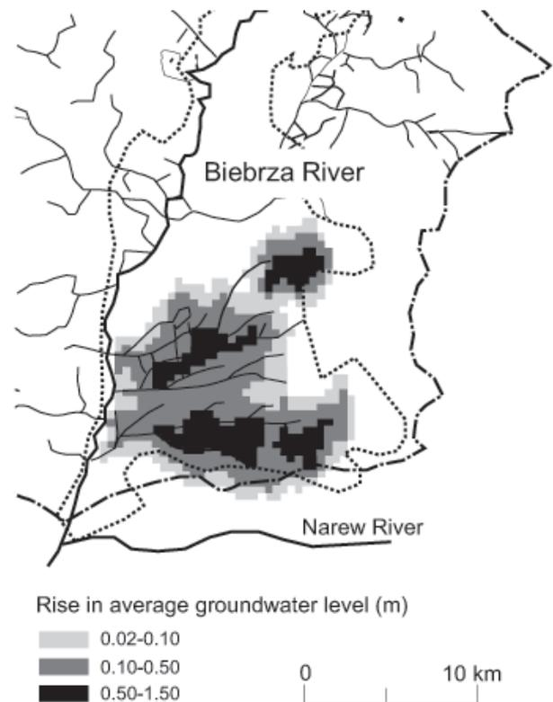
Fig. 5. Rise in average groundwater levels in summer for scenario 1 (damming ditches).
