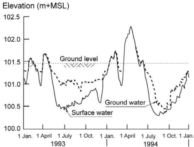
Fig. 6. Simulated groundwater and surface water levels during 1993 and 1994 for node 6633 (for location of node see Fig. 4).
