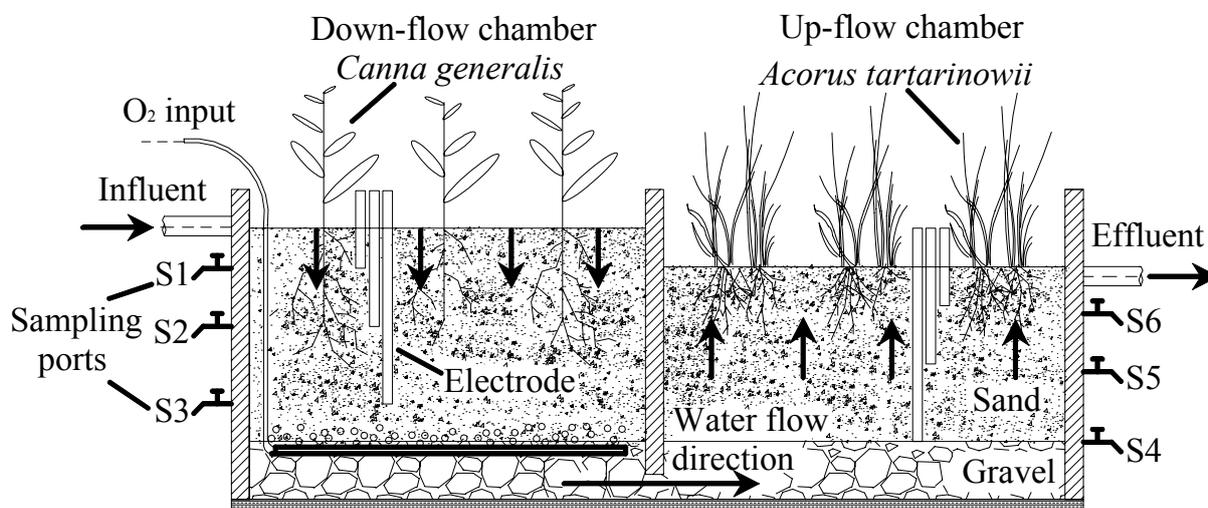
Fig. 1. Section view of aerated integrated vertical-flow constructed wetland.
