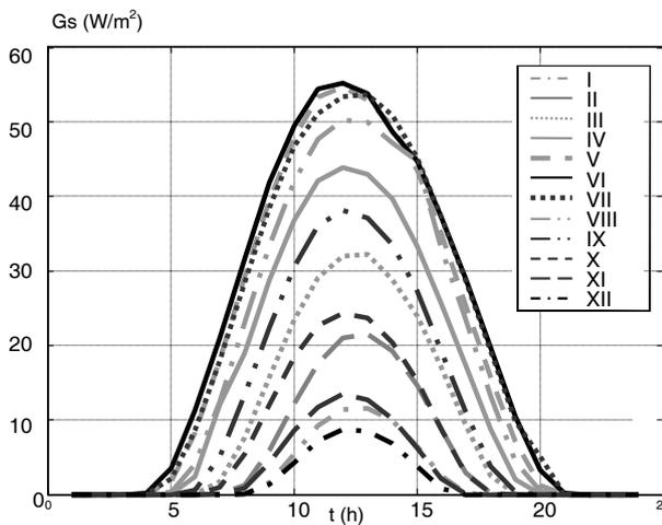
Fig. 1. Distribution of solar irradiance during averaged days for every month of a year for horizontal surfaces in Warszawa.
