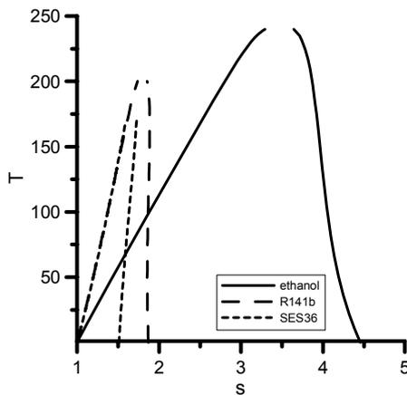
Fig. 2. T-s diagram for considered fluids calculated using Refprop 8.0.
