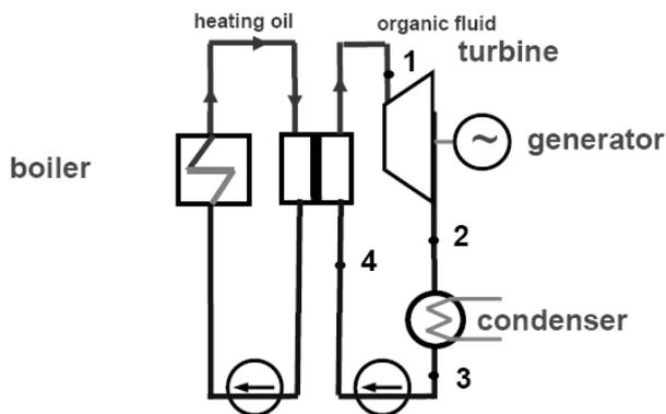
Fig. 3. Schematic of thermodynamic Rankine cycle of micro CHP.
