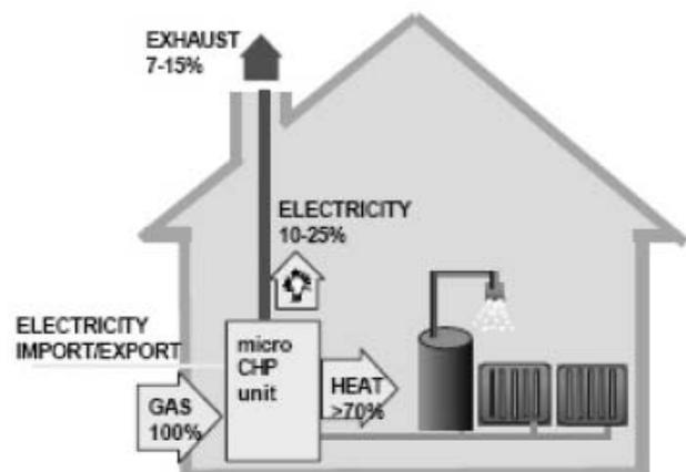
Fig. 1. General schematic of a micro CHP.
