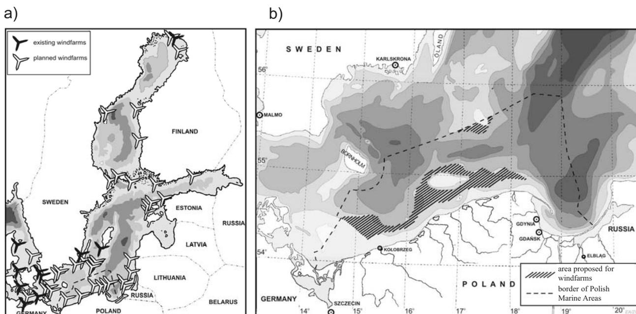
Fig. 5. a) Planned wind energy farms in the Baltic Sea. b) Areas considered for energy farm construction in Polish Marine Areas.
