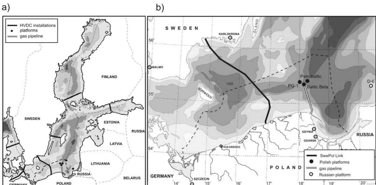
Fig. 4. a) Location of energy transmission lines in the Baltic Sea. b) The *SwePol Link* transmission line.
