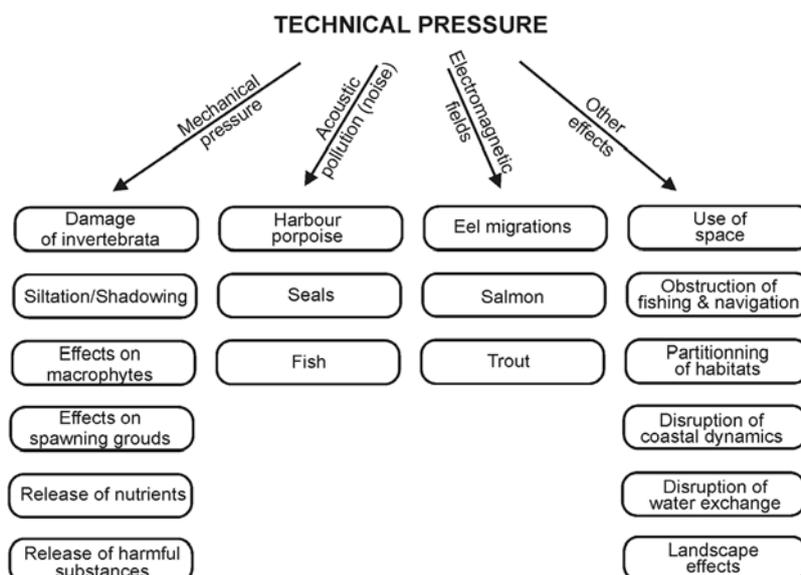
Fig. 6. Pressures of construction works.
