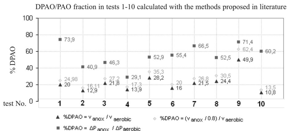
Fig. 4. Percent share of DPAO in PAO calculated with the literature published methods using 10 phosphorus uptake batch tests.
