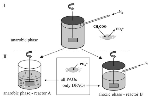
Fig. 1. The phosphorus uptake batch test procedure.
