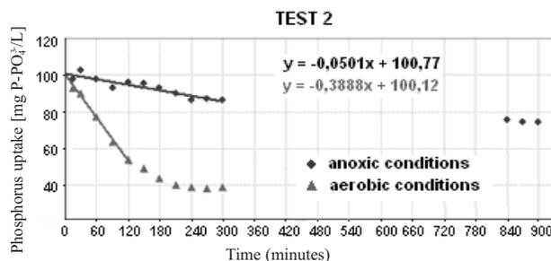
Fig. 3. Changes in orthophosphate concentrations under aerobic and anoxic conditions in the test No. 2.
