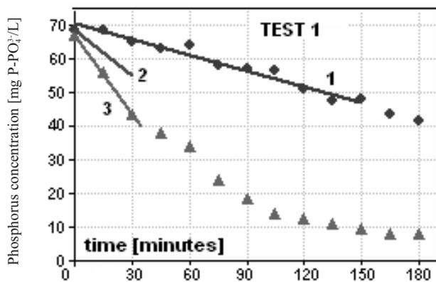
Fig. 5 Graphical representation of the measured phosphorus uptake rate under anoxic conditions (1) and the theoretical rate (2), at which the two discussed DPAO fraction estimations would have produced the same results. Curve 3 corresponds to orthophosphates uptake under aerobic conditions.
