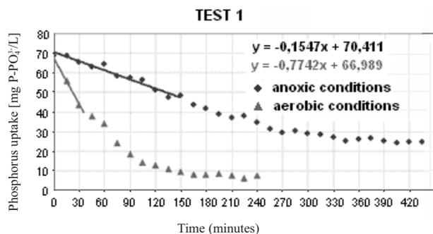
Fig. 2. Changes in orthophosphate concentrations under aerobic and anoxic conditions in the test No. 1.
