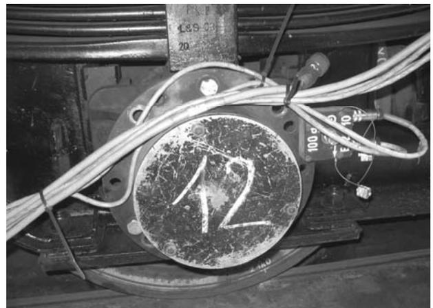
Fig. 3. Measurements of acceleration vibrations on the vehicle axle box.
