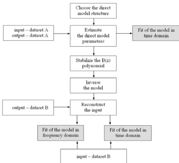
Fig. 2. Block diagram of the inversion procedure of a linear model.
