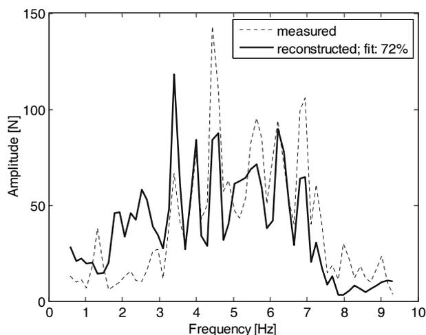
Fig. 4. Results of load reconstruction presented in the frequency domain at the left side of the vehicle in the vertical direction obtained with the use of ARX(33,29,1).
