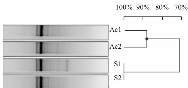
Fig. 5. Digitized profiles and dendrogram showing clustering analyses of activated sludge, obtained with polymerase chain reaction RAPD from the target DNA extracted by the freeze and thaw method.
