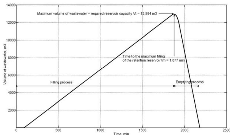
Fig. 7. Determination of the maximum storage reservoir capacity.
