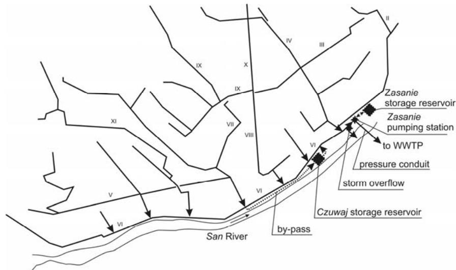
Fig. 4. Schematic diagram of sewage network of the Zasanie residential quarter in Przemyśl with Zasanie and Czuwaj retention reservoirs planned for construction.
