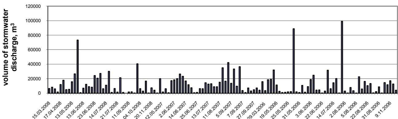
Fig. 3. Combined sewage volumes discharged from storm overflow upstream of the Zasanie Sewage Pumping Station, in 2006-08.
