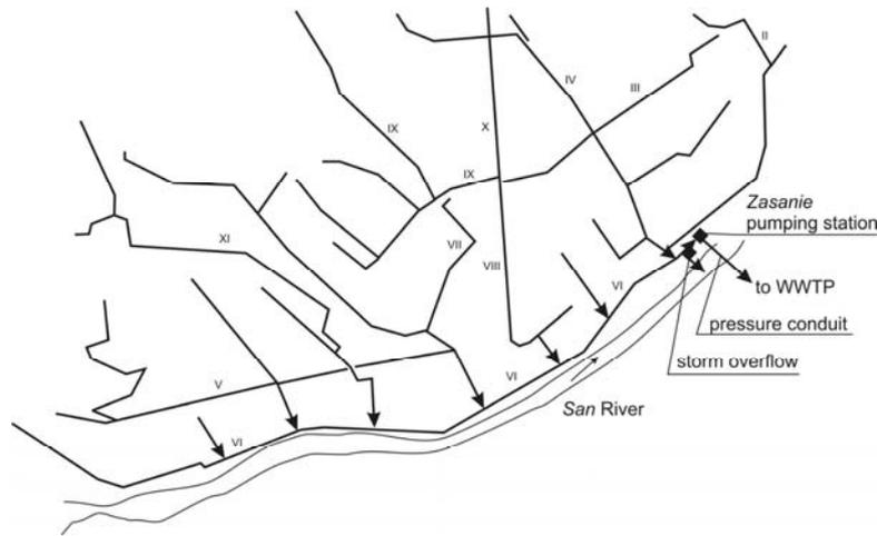
Fig. 2. Schematic diagram of the sewage system existing in the Zasanie district of the town of Przemysł.
