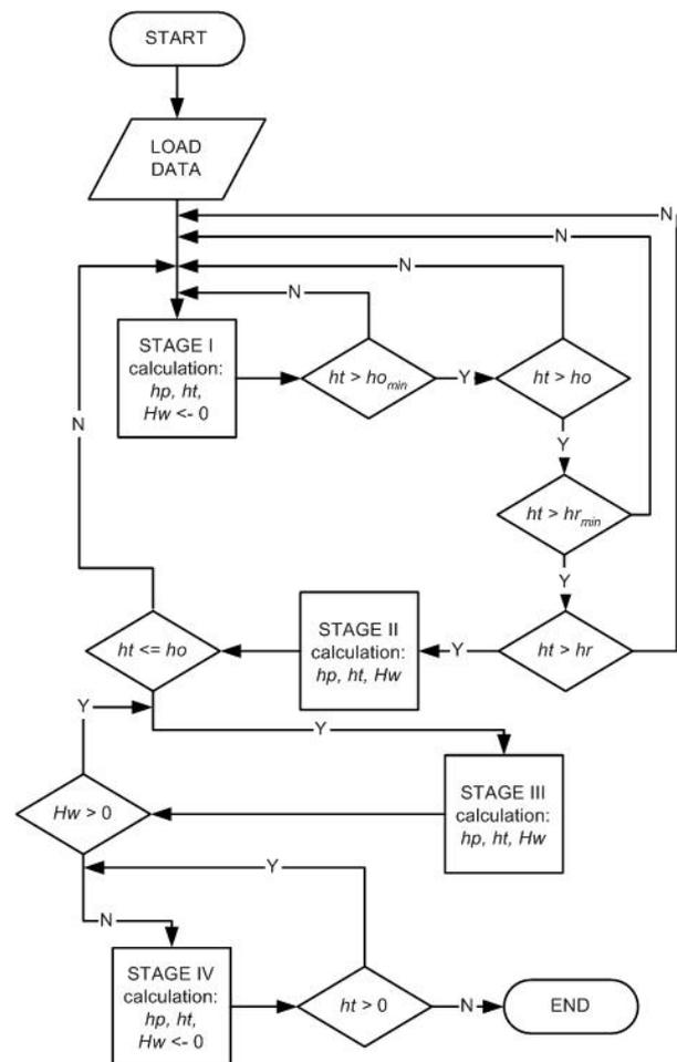
Fig. 6. Algorithm of PSZ simulation program.
