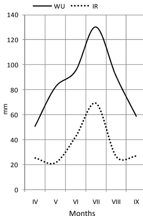
Fig. 2. Water use from the soil layer of controlled moisture (WU) and irrigation requirements (IR) at forest nursery Białe Błota near Bydgoszcz, acc. to Pierzgalski et al. [16], mean for 2005-07 (mm).
