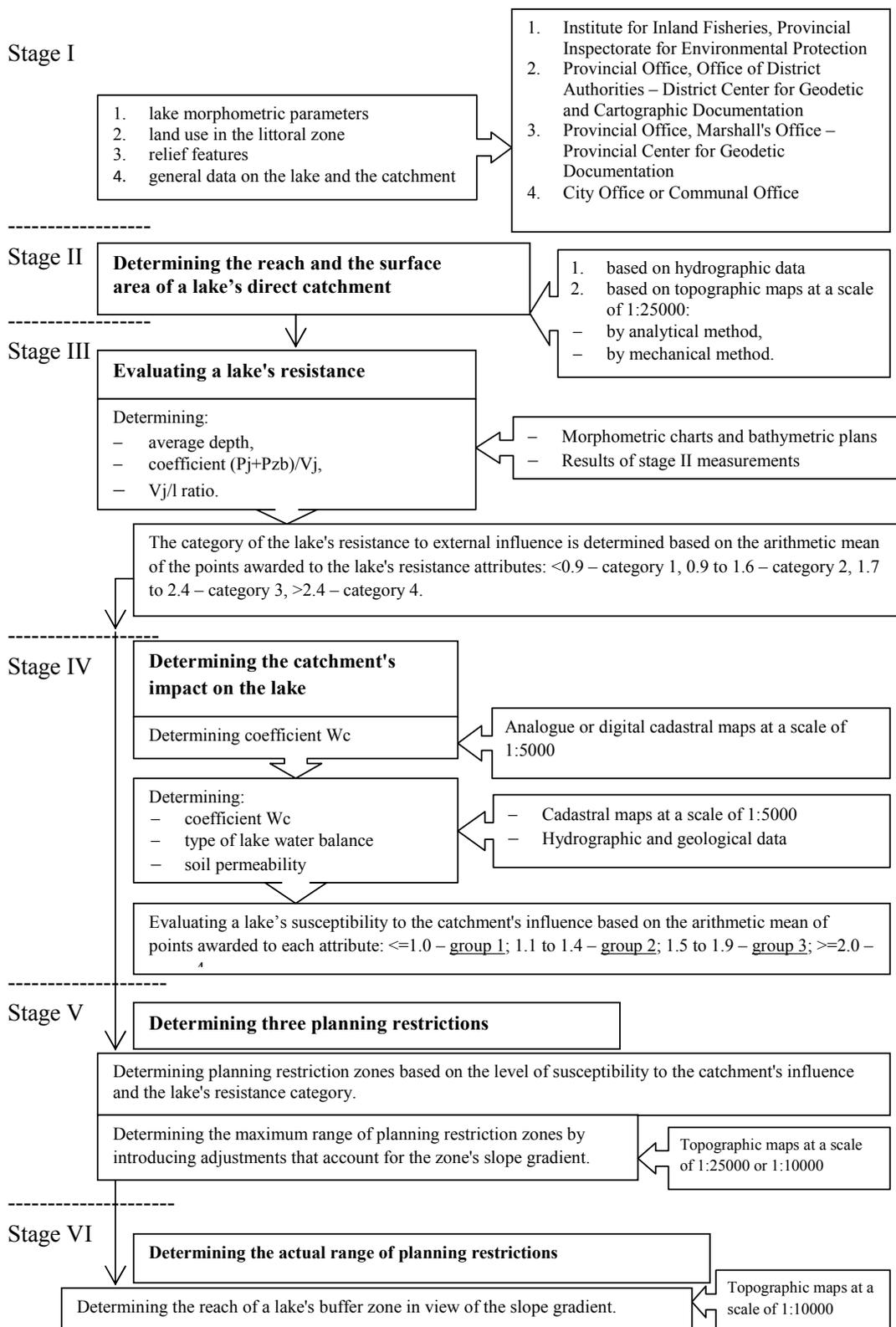
Fig. 4. Schematic presentation of the process of developing limnological restrictions.
