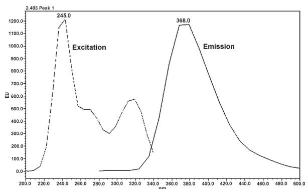
Fig. 2. Fluorescence spectra of AMO+AccQ-Fluor product. Excitation spectrum with emission at 368 nm, emission spectrum with excitation at 245 nm.
