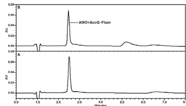
Fig. 5. Chromatograms obtained for AMO pure substance+AccQ-Fluor (A) and AMO suspension extract+AccQ-Fluor (B) derivatives recorded at UV detection.
