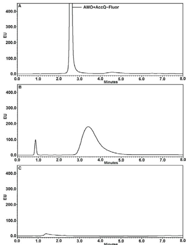
Fig. 3. Chromatograms recorded, after derivatization reaction with AccQ-Fluor reagent, for AMO without degradation (A) and for AMO subjected to the chemical degradation using 1 M HCl (B) and 1 M NaOH (C).
