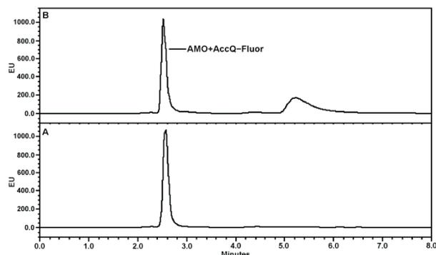
Fig. 4. Chromatograms obtained for AMO pure substance+AccQ-Fluor (A) and AMO suspension extract+AccQ-Fluor (B) derivatives recorded at fluorescence detection.
