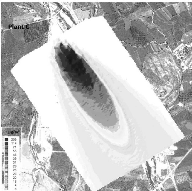
Fig. 4. SO<sub>2</sub> concentration distribution map for Plant C.
