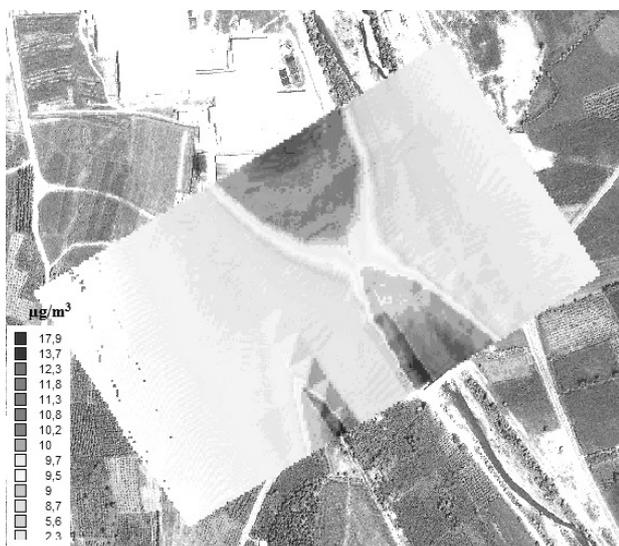
Fig. 11. SO<sub>2</sub> concentration distribution map of intersection area for plants B and A.
