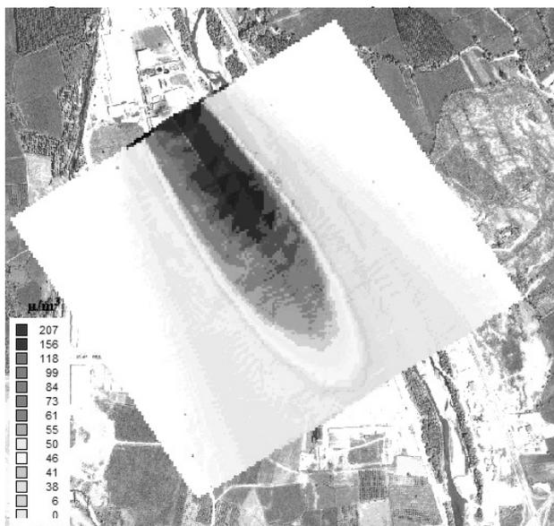
Fig. 10. SO<sub>2</sub> concentration distribution map of emission plume intersection areas for plants C and B.
