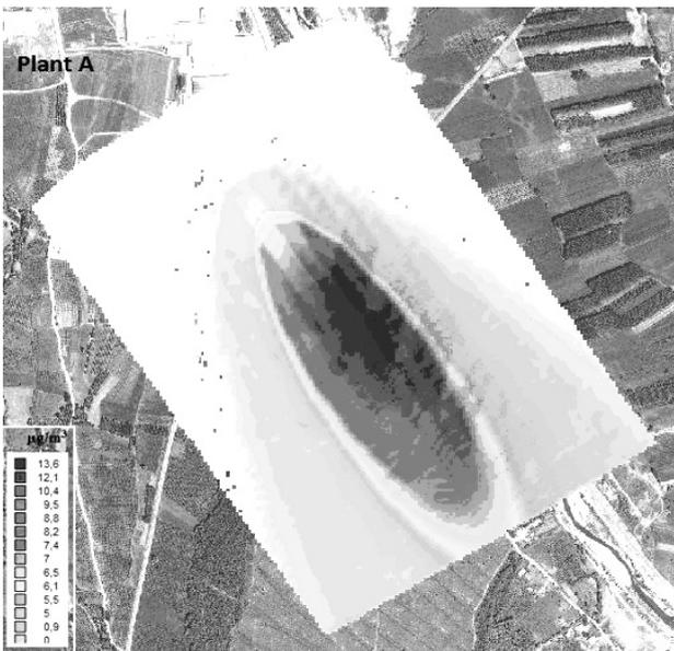
Fig. 8. SO<sub>2</sub> concentration distribution map for Plant A.
