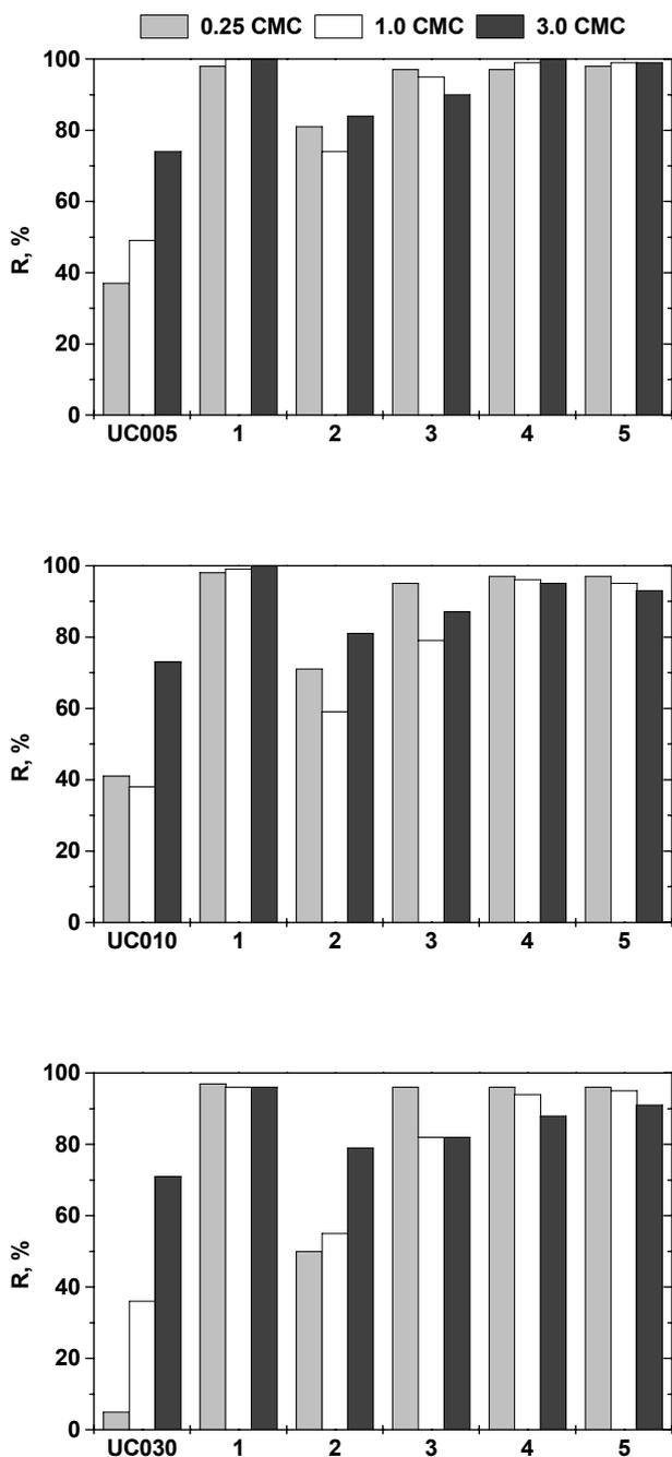
Fig. 5. Surfactant removal efficiency (%) in a sequential ultra-filtration ion exchange purification system (membrane material: cellulose, contact time: 20 min., resin dose: 20 cm<sup>3</sup>/dm<sup>3</sup>, 1 – MIEX<sup>®</sup>, 2 – A100, 3 – A200, 4 – A400, 5 – SBW).
