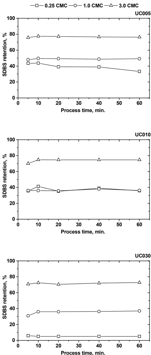
Fig. 3. Surfactant removal efficiency (%) during the ultrafiltration process (membrane material: cellulose).
