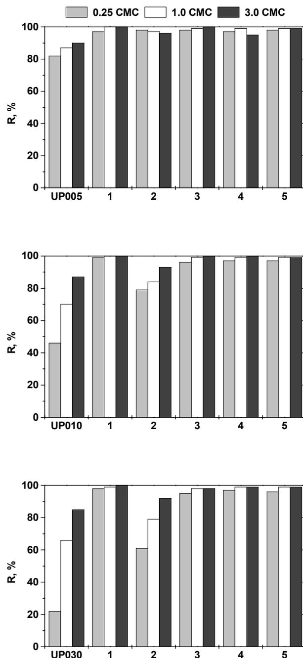
Fig. 4. Surfactant removal efficiency (%) in a sequential ultrafiltration – ion exchange purification system (membrane material: polyethersulfone, contact time: 20 min., resin dose: 20 cm<sup>3</sup>/dm<sup>3</sup>, 1 – MIEX<sup>®</sup>, 2 – A100, 3 – A200, 4 – A400, 5 – SBW).
