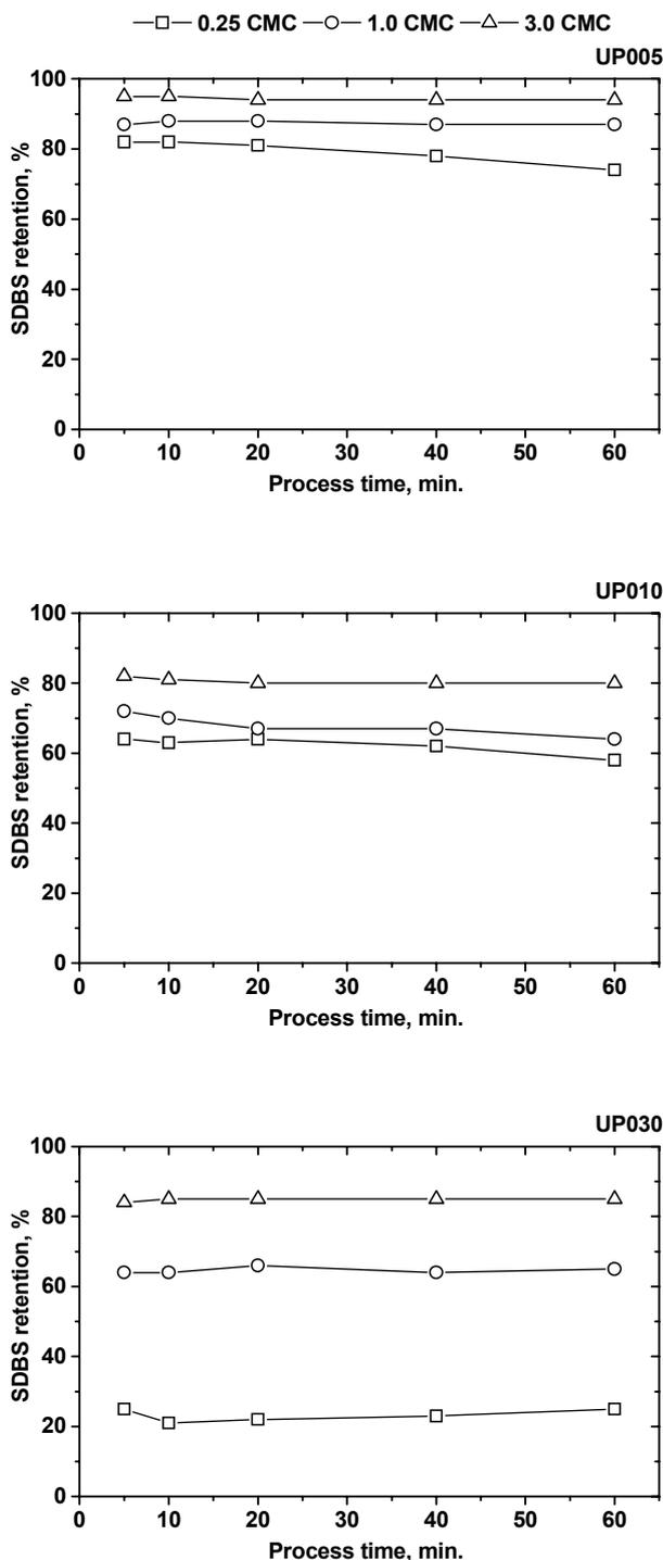
Fig. 2. Surfactant removal efficiency (%) during the ultrafiltration process (membrane material: polyethersulfone).
