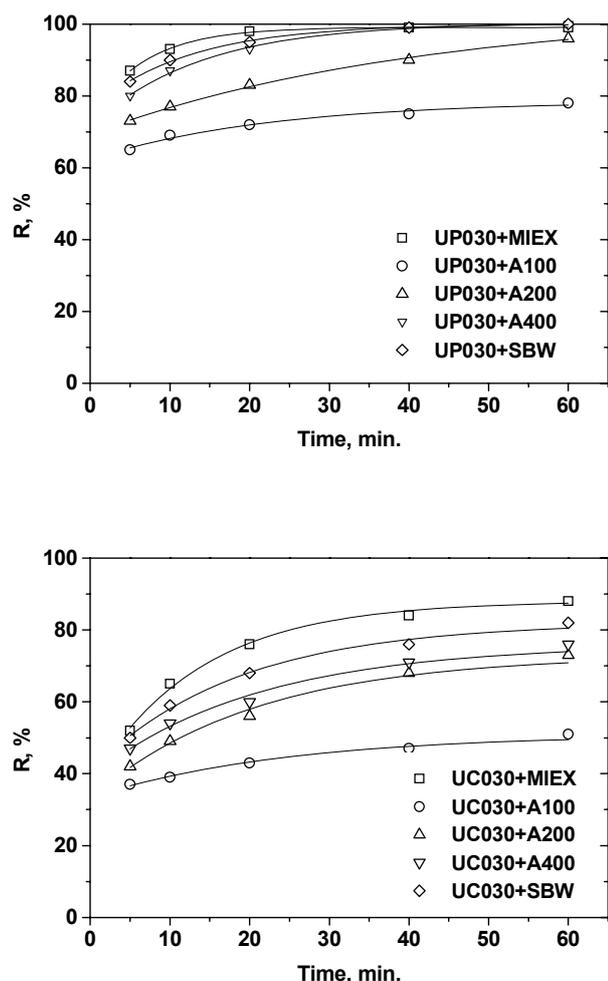
Fig. 6. Surfactant removal efficiency (%) in a sequential ultrafiltration – ion exchange purification system as a function of contact time (resin dose: 10 cm<sup>3</sup>/dm<sup>3</sup>, surfactant concentration: 1.0 CMC).
