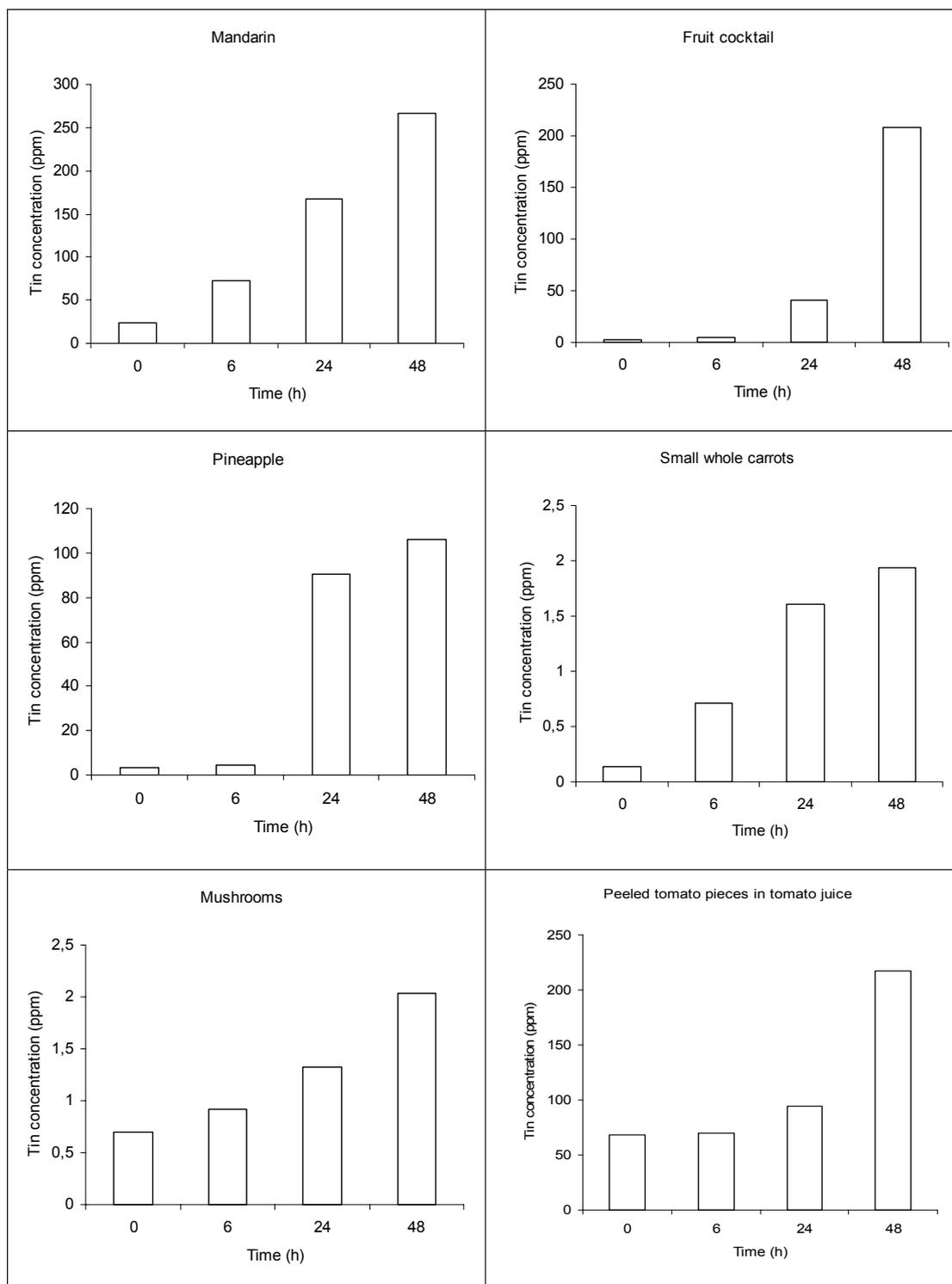
Fig. 1. Effects of standing in an opened can (at 20°C) on tin content in syrup.
