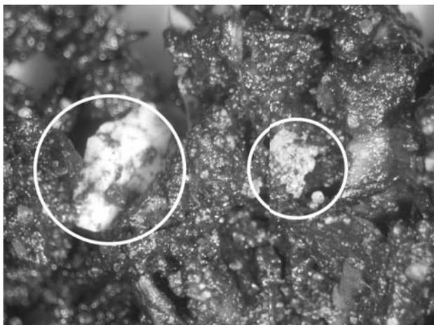
Fig. 7. Ground peroxide vulcanizate of polybutadiene rubber among the particles of vermicompost substratum (Photo. M. A. Józwiak).
