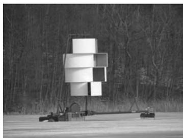
Fig. 2. The scheme of the pulverizer operation [after 21, changed] and photography of the pulverising aerator with vertical Savonius turbine on Lake Göreckie.
