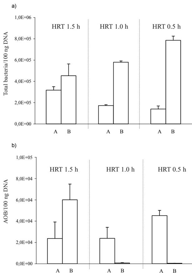
Fig. 1. The number of total bacteria (a) and AOB (b) at three different HRTs in modes A and B.
