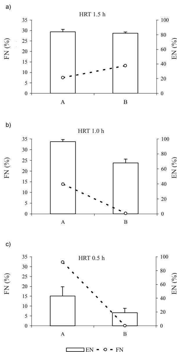
Fig. 2. Nitrification efficiency (EN) and percentage of AOB in activated sludge (FN) in modes A and B; a) HRT 1.5 h, b) HRT 1 h, c) HRT 0.5 h; nitrification efficiency (EN): the ratio of total Kjeldahl nitrogen removed minus nitrogen used for biomass synthesis to total Kjeldahl nitrogen in the influent.
