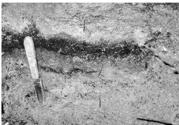
Fig. 3. Typical soil profile along the experimental transect with a surface greyish layer of wind-deposited tailings, dark Ah horizon, and bottom brown-orange Bw horizon.
