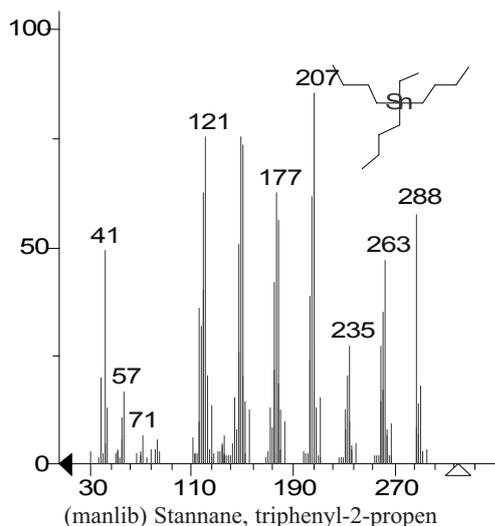
Fig. 6. Mass spectra of TBT derivatives TBT: 207.
