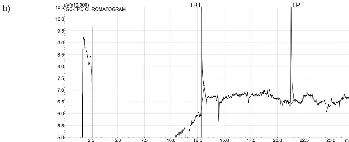
Fig. 2. a) GC-MS TOF chromatograms for the analysis of organotin in reference sediment, sample and mixture TBT: 11.42; b) GC-FPD showing chromatogram of reference standards.
