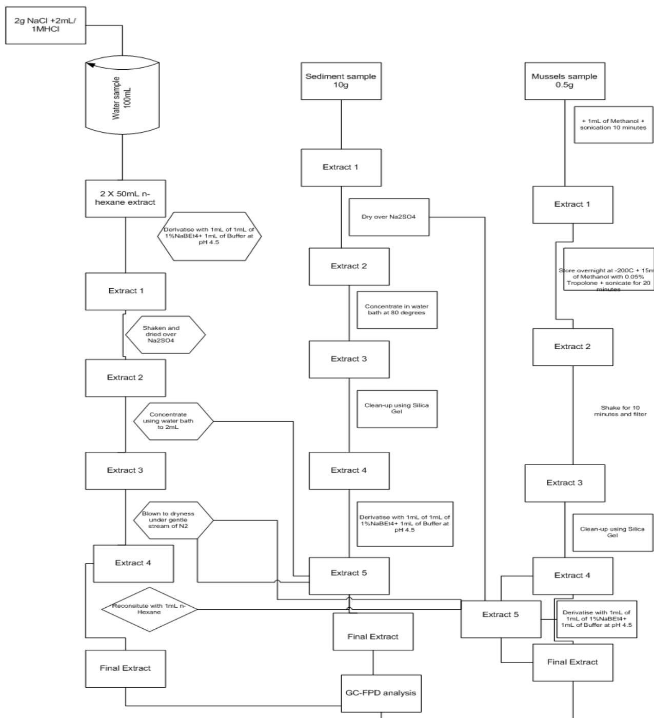
Fig. 9. A schematic diagram of overall extraction procedures for water, sediment, and mussel samples.
