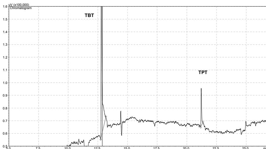
Fig. 8. GC-FPD chromatogram for organotin compounds in real sediment samples from Cape Town harbor.
