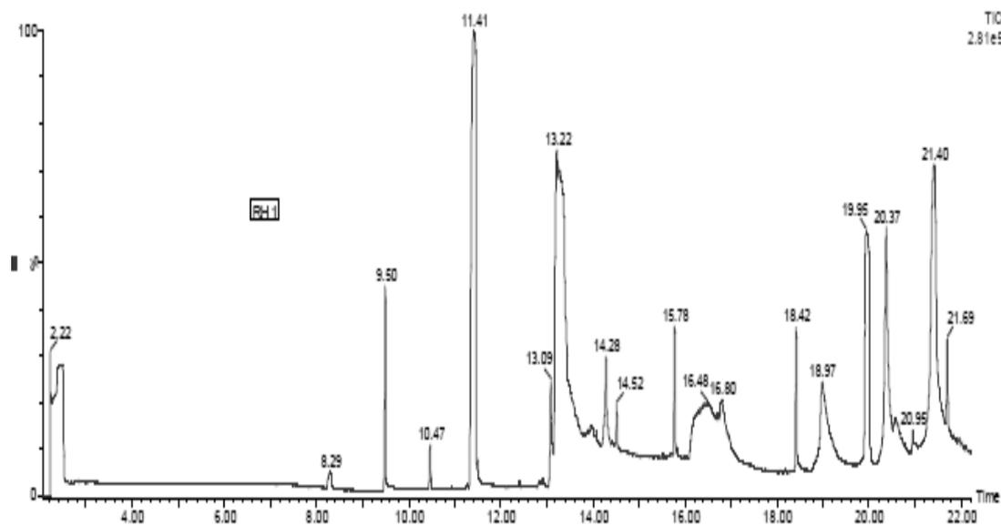
Fig. 4. Chromatogram of organotins in the spiked water sample taken from the laboratory recorded from GC-MS – TOF. TBT: 11, 41; TPT: 21, 40
