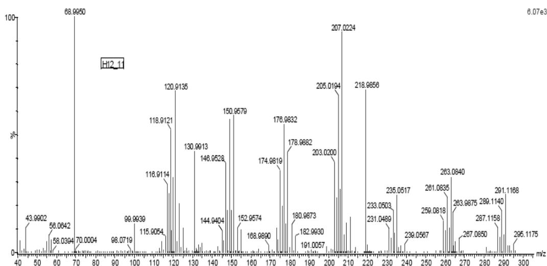
Fig. 5. Mass spectra of organotins in the real water samples from Cape Town harbor. TBT: 207.0224; TPT: 120.9135
