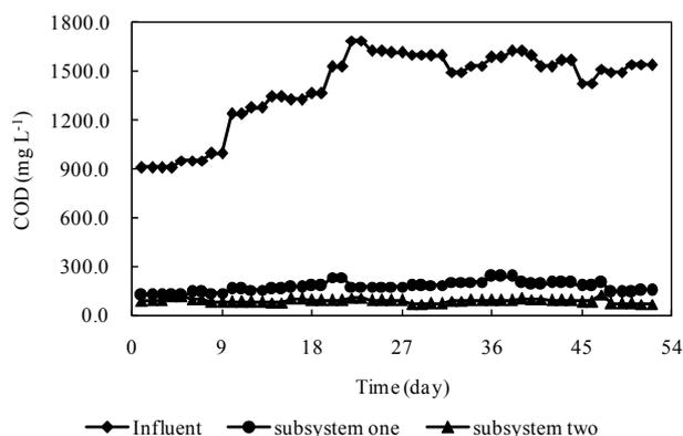
Fig. 2. COD concentration of influent and the two subsystem effluents.
