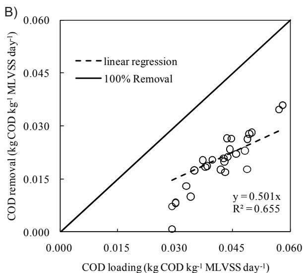
Fig. 3. COD loading and removal rates of two subsystems.
