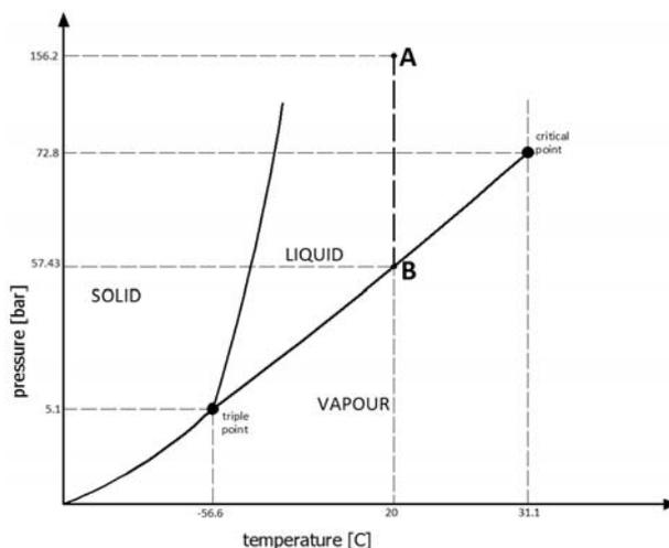
Fig. 2. Phase diagram of carbon dioxide.
