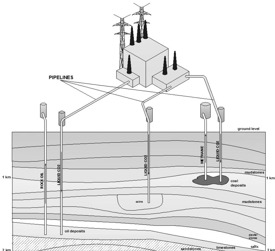
Fig. 1. Possibilities of underground CO<sub>2</sub> storage.
