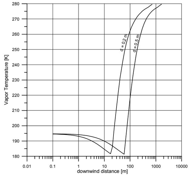
Fig. 4. Change in CO<sub>2</sub> temperature depending on distance from the outflow.
