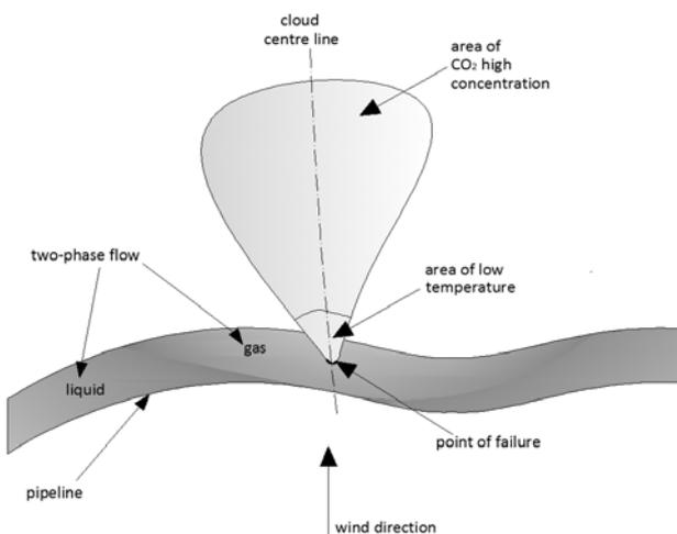
Fig. 3. Gas outflow from the damaged pipeline.
