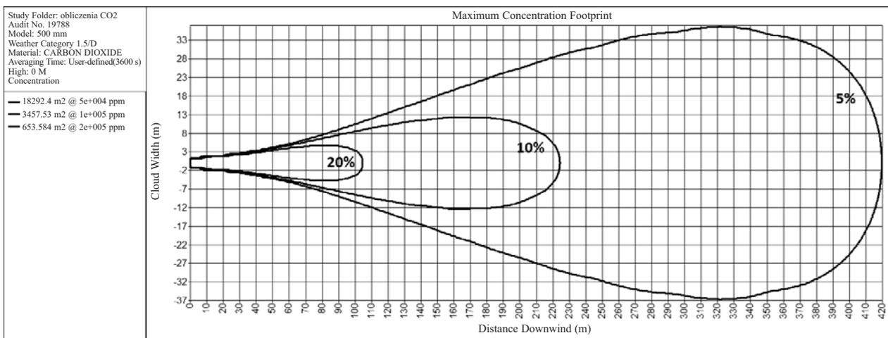
Fig. 7. CO<sub>2</sub> concentration areas for a 0.5 m diameter pipeline.
