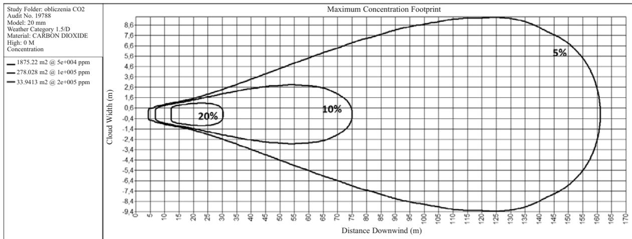
Fig. 6. CO<sub>2</sub> concentration areas for a 0.2 m diameter pipeline.
