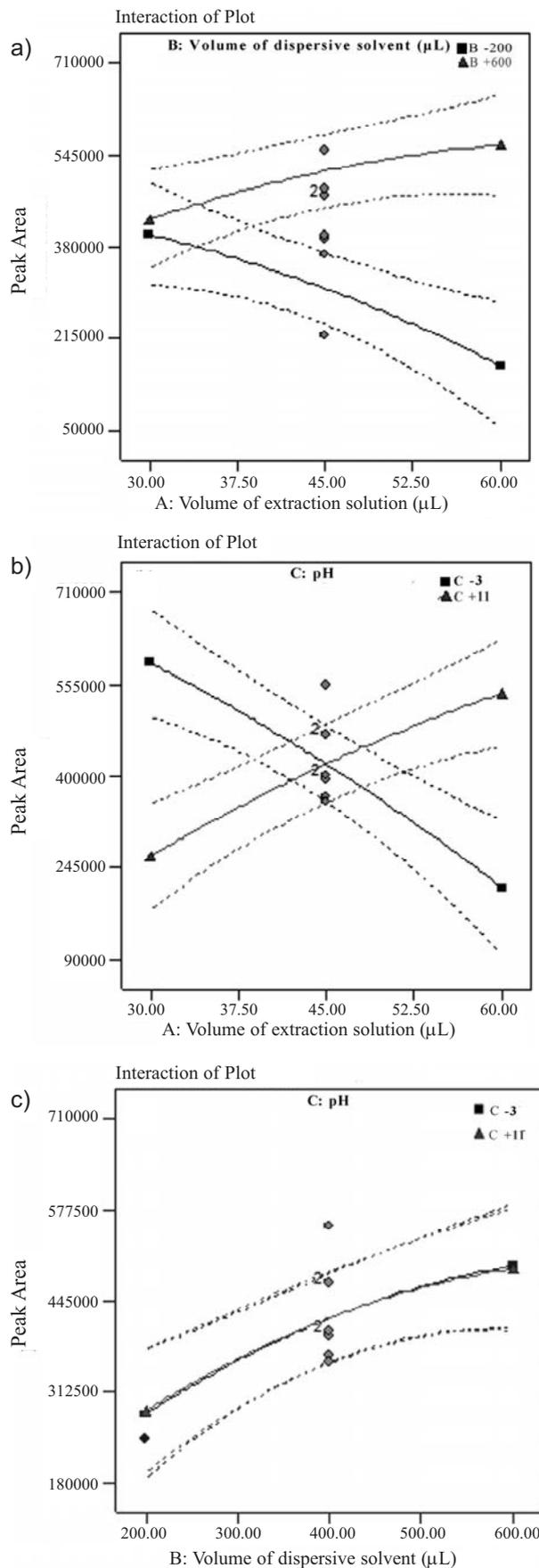
Fig. 3. Two-factor interaction and their effects on efficiency: (a) volume of extraction solvent and volume of dispersive solvent, (b) volume of extraction solvent and pH, and (c) volume of dispersive solvent and pH.
