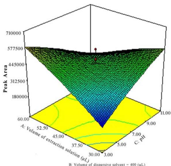
Fig. 5. Response surface curve showing the predicted response as an interaction function of volume of extraction solvent ranging from 30 to 60  $\mu\text{L}$ , and pH ranging from 3 to 11 by holding the volume of dispersive solvent at its central level (400  $\mu\text{L}$ ).
