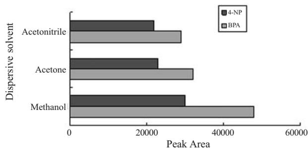
Fig. 1. Effects of different dispersive solvents on the efficiencies of enrichment of BPA and 4-NP.
