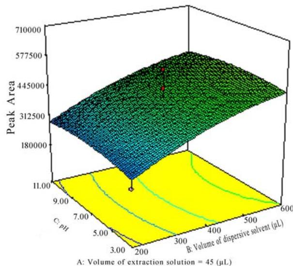
Fig. 6. Response surface curve showing the predicted response as an interaction function of the volume of dispersive solvent ranging from 200 to 600  $\mu\text{L}$  and pH ranging from 3 to 11 by holding the volume of extraction solvent at its central level (45  $\mu\text{L}$ ).
