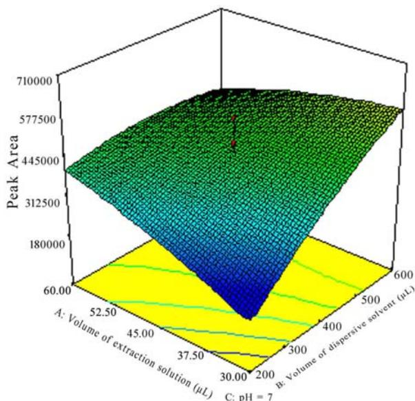
Fig. 4. Response surface curve showing the predicted response as an interaction function of volume of extraction solvent ranging from 30 to 60  $\mu\text{L}$  and volume of dispersive solvent ranging from 200 to 600  $\mu\text{L}$  by holding pH at its central level (7).
