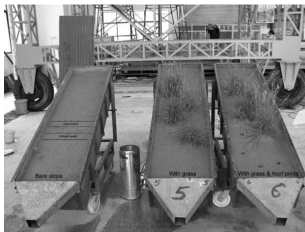
Fig. 1. Photos of three kinds of microtopography of soil surface and experimental seed distribution (H1-5 shows the position of the hoof prints).
