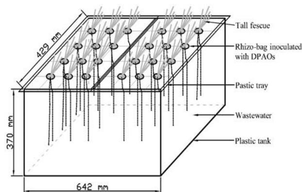
Fig. 1. Schematic diagram of stereo floating beds inoculated with denitrifying polyphosphate-accumulating microorganisms (DPAOs).
