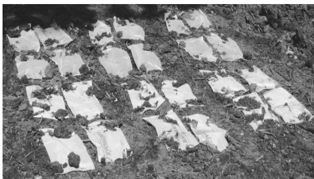
Fig. 1. The arrangement of samples (one of two layers) in the compost heap.
