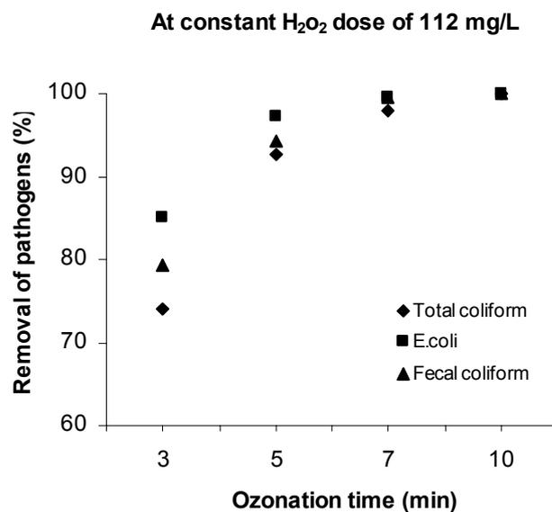
Fig. 5. The performance (%) of the O<sub>3</sub>/H<sub>2</sub>O<sub>2</sub> system for the removal of pathogens.
