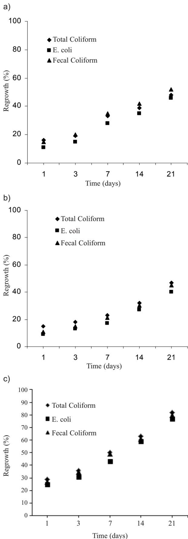
Fig. 9. Regrowth (%) of pathogens in UASB effluent disinfected with UV irradiation for 3 minutes in the (a) presence of light, (b) absence of light, and (c) presence of nutrients.
