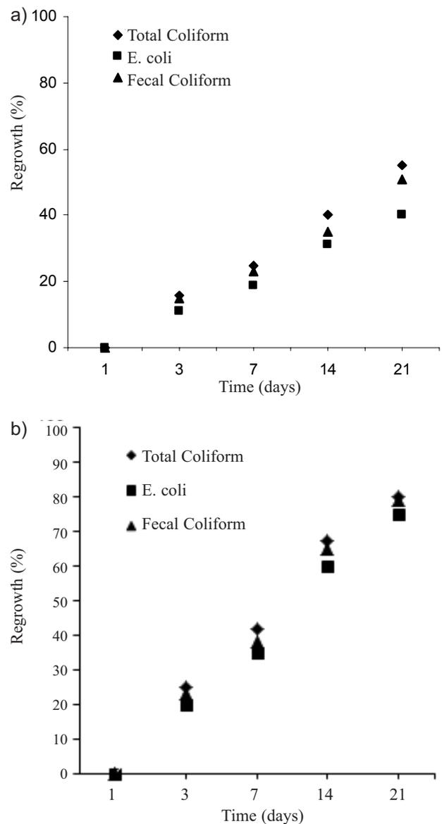
Fig. 10. Regrowth (%) of pathogens in UASB effluent disinfected with UV irradiation for 7 minutes at (a) 15°C and (b) 35°C.
