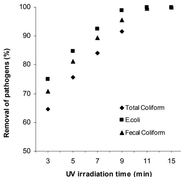
Fig. 2. The pathogen removal efficiency (%) of UV irradiation.
