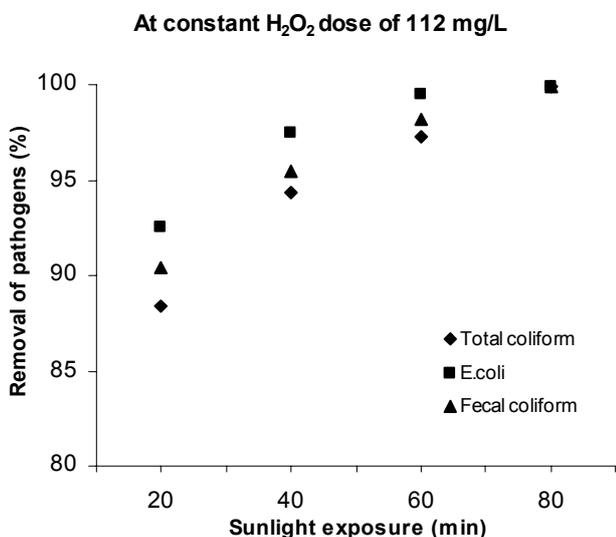
Fig. 4. The inactivation efficiency (%) of the H<sub>2</sub>O<sub>2</sub>/sunlight system.
