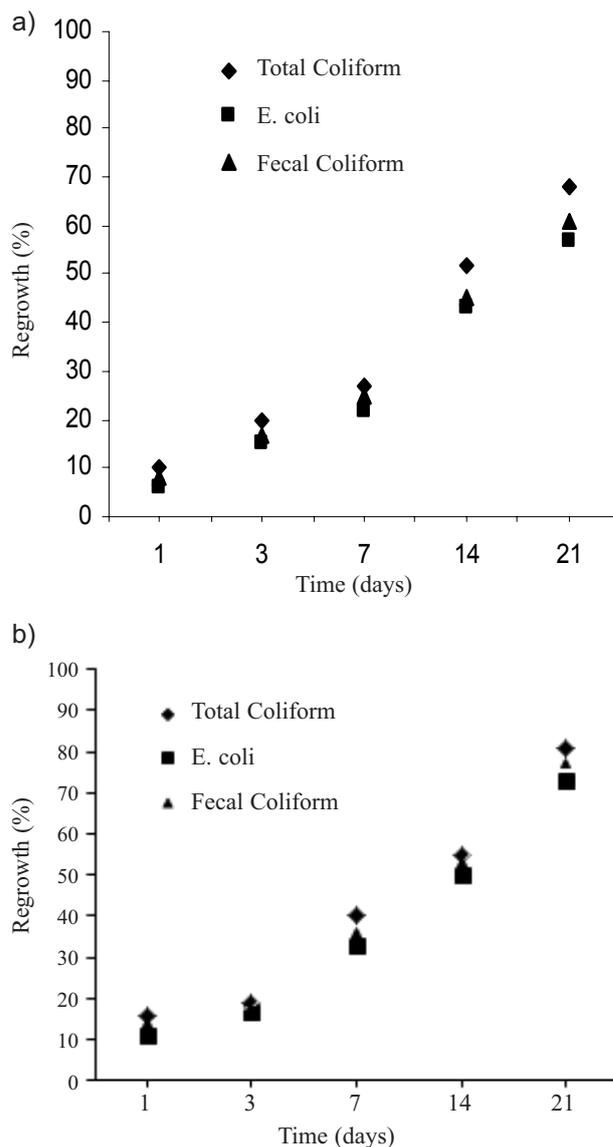
Fig. 8. Regrowth (%) of pathogens in UASB effluent disinfected with UV irradiation for 3 min at: (a) 15°C and (b) 35°C.
