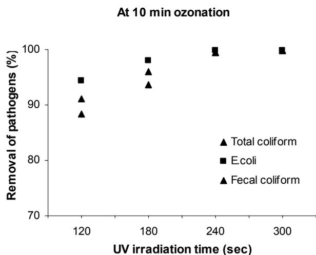
Fig. 7. The removal of pathogens by the O<sub>3</sub>/UV system in effluents.
