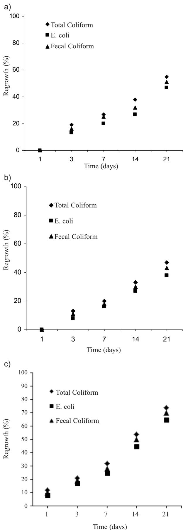
Fig. 11. Regrowth (%) of pathogens in UASB effluent disinfected with UV irradiation for 7 minutes in the (a) presence of light, (b) absence of light, and (c) presence of nutrients at 35°C.
