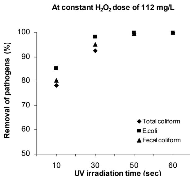
Fig. 6. The inactivation efficacy (%) of the H<sub>2</sub>O<sub>2</sub>/UV system.
