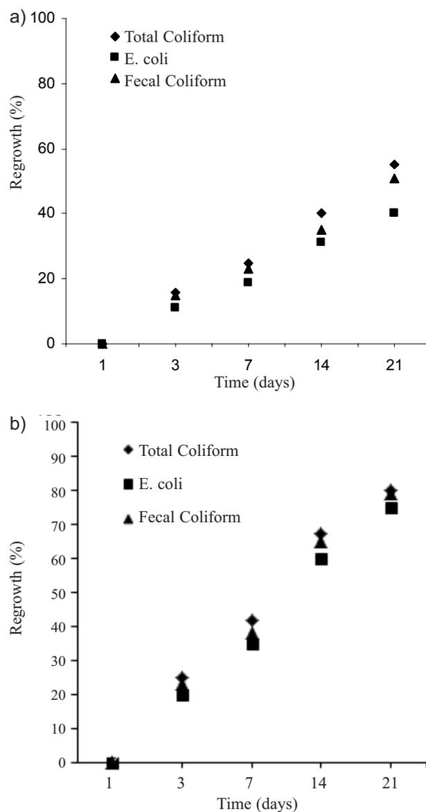
Fig. 10. Regrowth (%) of pathogens in UASB effluent disinfected with UV irradiation for 7 minutes at (a) 15°C and (b) 35°C.
