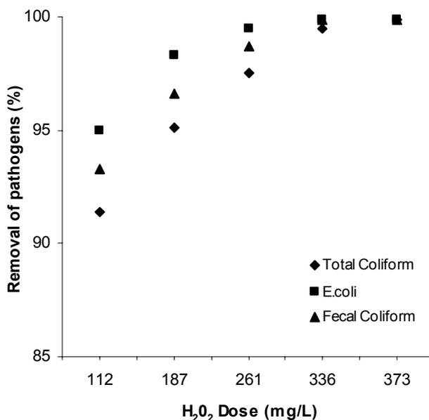
Fig. 3. The influence of H<sub>2</sub>O<sub>2</sub> dose on its inactivation efficiency (%).
