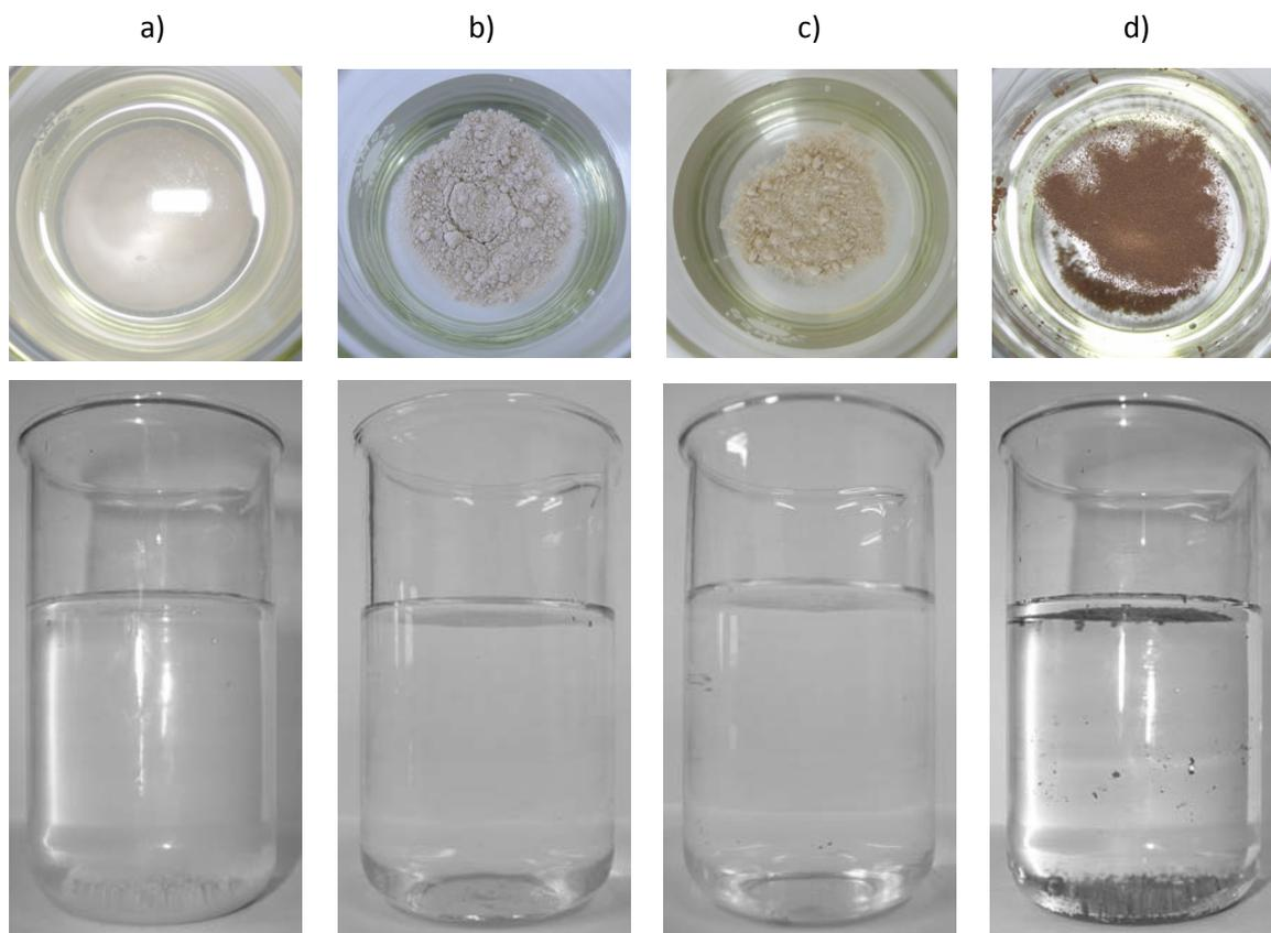
Fig. 1. The “floating on water” test. Limestone meal: a) raw, b) modified in stearic acid vapours, c) modified by mixing with the Sarsil® H-15 preparation, d) modified with the Bitumen Voranstrich preparation.
