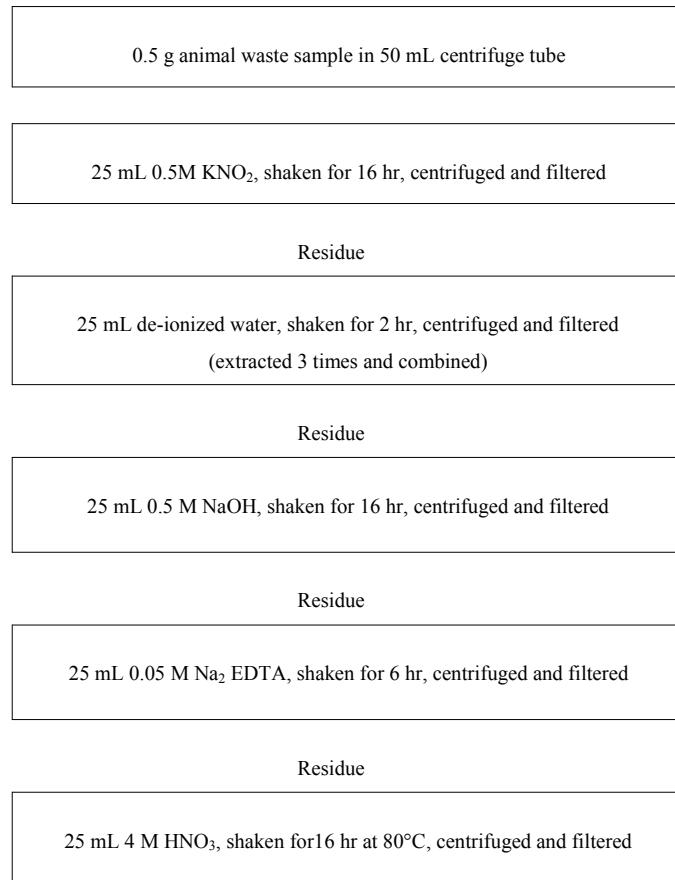
Fig. 1. Schematic diagram of sequential fractionation of trace elements.
