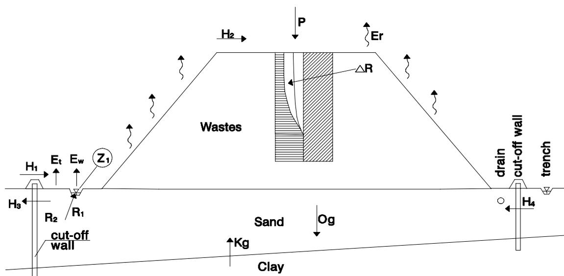
Fig. 2. Scheme of Radiowo landfill water balance components [8]. (P – precipitation,  $H_2$  – surface flow,  $Er$  – evaporation from slopes and landfill crest,  $\Delta R$  – effective capability of retention,  $Kg$  – capillary rise,  $H_4$  – ground flow,  $Og$  – ground leachate,  $E$  – evapotranspiration).
