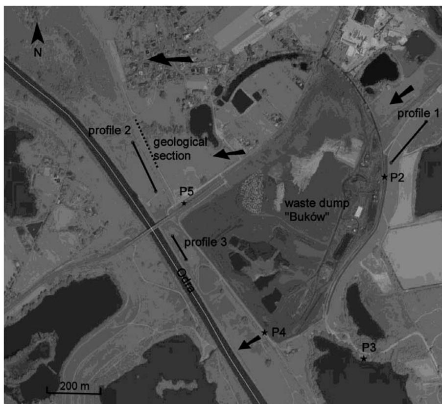
Fig. 1. Location of the survey area. Arrows indicate direction of underground water flow. (accor. Google Earth.com).
