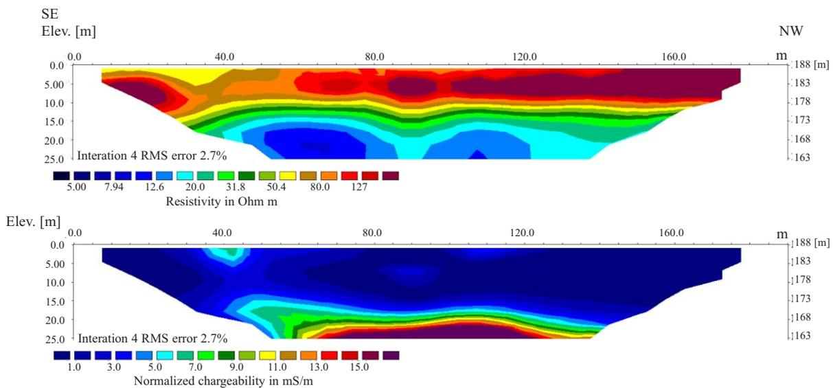
Fig. 4. Inverted resistivity and normalized chargeability values obtained for profile 2.
