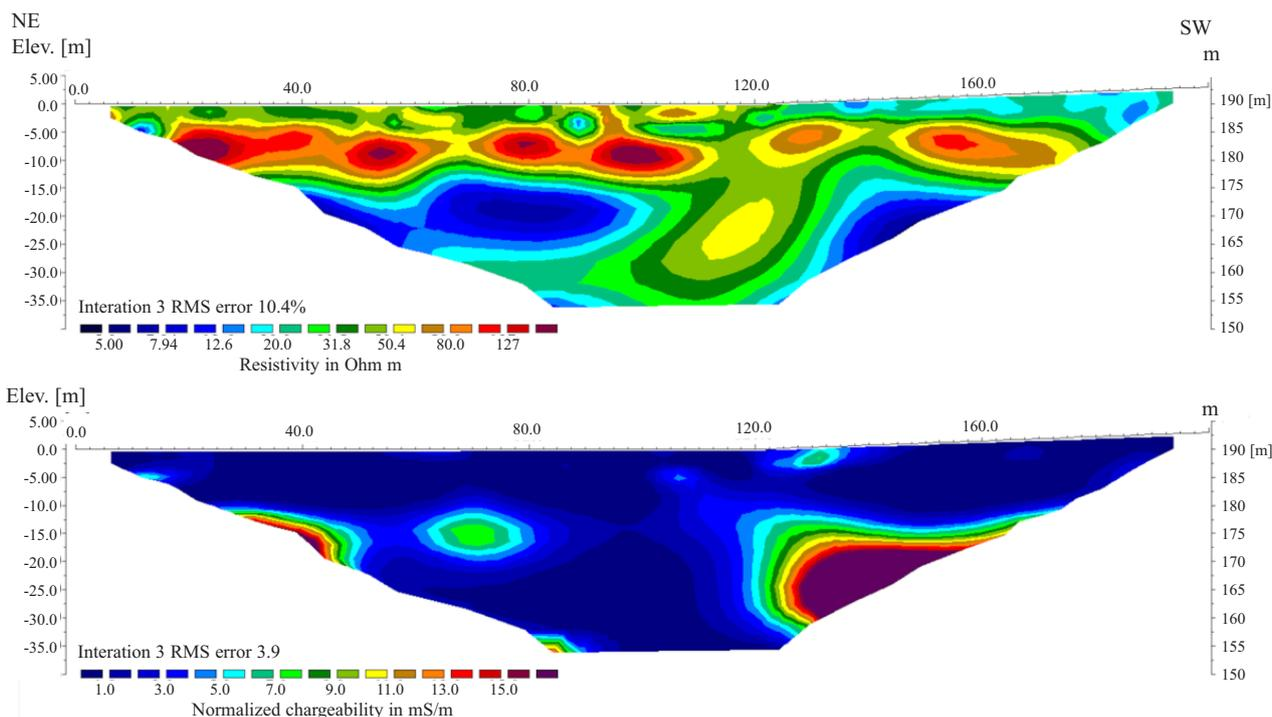
Fig. 3. Inverted resistivity and normalized chargeability values obtained for profile 1.
