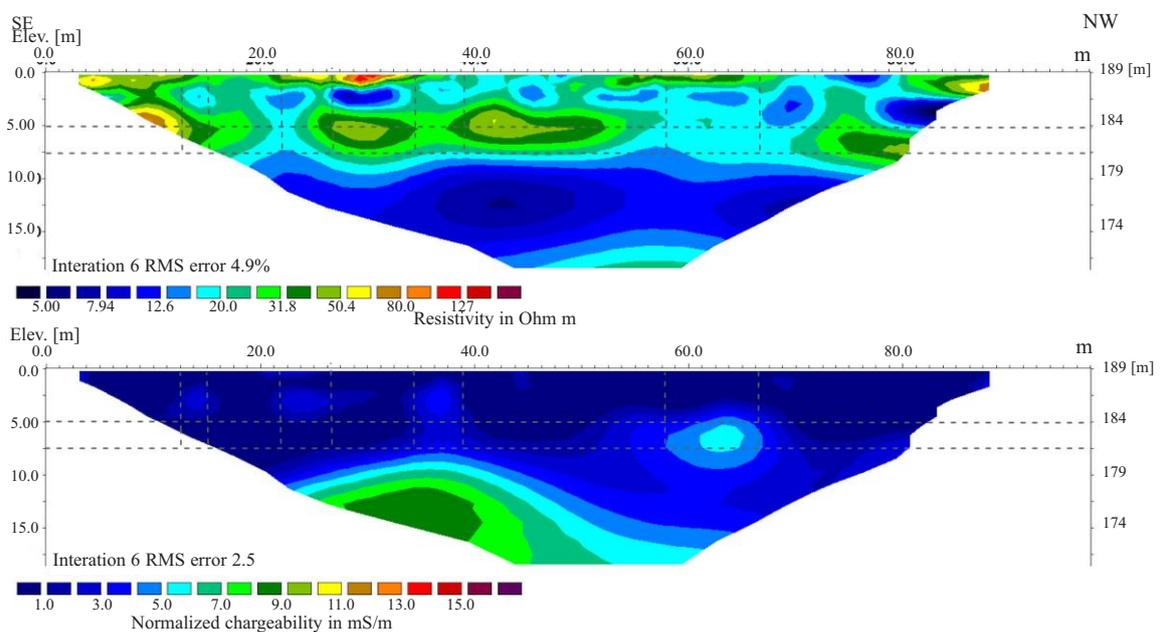
Fig. 5. Inverted resistivity and normalized chargeability values obtained for profile 3.
