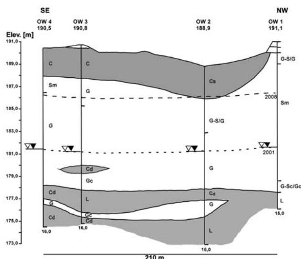
Fig. 2. The geological section of the investigated area. G – gravel, G-S – sand-gravel, Gc – clayey gravel, Sc – coarse sand, Sm – medium sand, C – clay, Cs – sandy clay, Cd – dusty clay, L – loam
