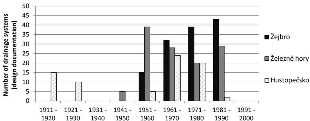
Fig. 7. Number of drainage measures implemented in the individual decades in the model localities; source: authors (vector layer created according to the design documentation).
