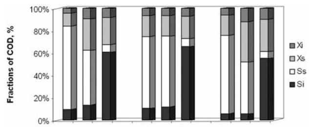
Fig. 5. COD fractions for small treatment plant in Zielniki during series I, II, III; 1 – inflow, 2 – septic tank effluent, 3 – outflow.
