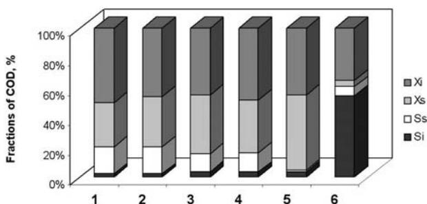
Fig. 7. COD fractions for municipal WWTP in Chwałkowo during series III; 1 – outlet from screen, 2 – outlet from grit chamber, 3 – inlet to defosfatation tank, 4 – outlet from defosfatation tank, 5 – outlet from aeration tank, 6 – outflow.
