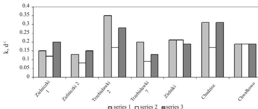
Fig. 11. Reaction rate  $k$ -coefficient for wastewater from investigated treatment in three series of research.
