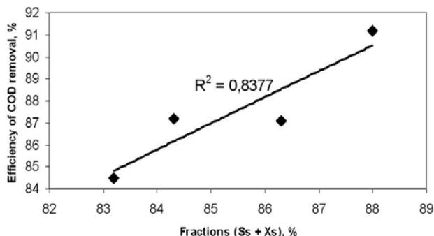
Fig. 10. Relationship between fraction of sum of  $S_s$  and  $X_s$  and efficiency of COD removal for small treatment plants in Zielniki and Chudzice.
