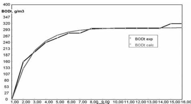
Fig. 2. Determination of  $k$  and  $BOD_{tot}$  using Polymath program.
