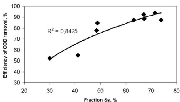
Fig. 8. Relationship between  $S_S$  fraction and efficiency of COD removal for individual treatment plants in Zielniczki and Trzebisławki.
