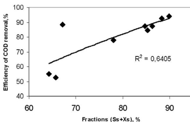
Fig. 9. Relationship between fraction of sum of  $S_S$  and  $X_S$  and efficiency of COD removal for individual treatment plant in Zielniczki and Trzebisławki.
