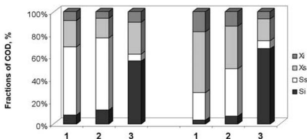
Fig. 6. COD fractions for small treatment plant in Chudzice during series I, II; 1 – inflow, 2 – septic tank effluent, 3 – outflow.
