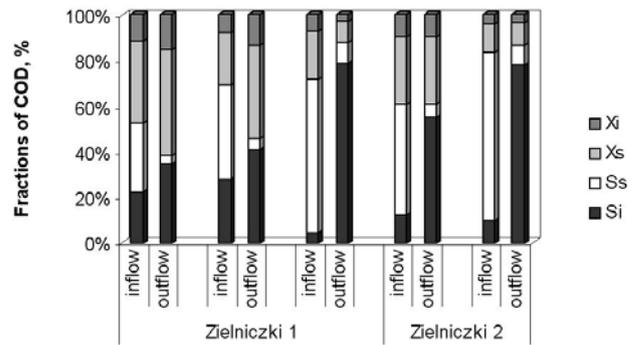
Fig. 3. COD fractions for individual treatment plants in Zielniczki during series I, II, III.
