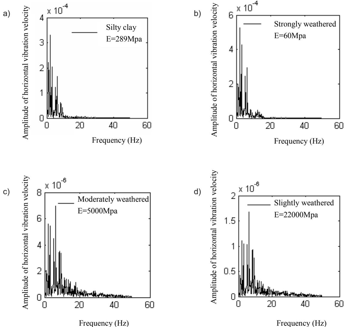
Fig. 7. Amplitude of horizontal vibration velocity 10 m from the center of the tunnel.
