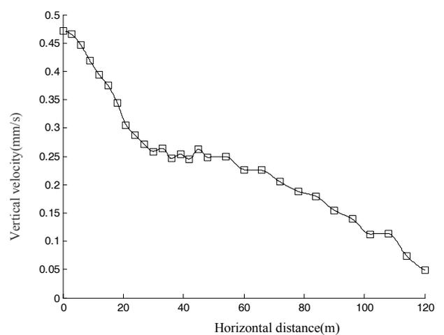
Fig. 24. Variation of vertical velocity amplitude with horizontal distance.
