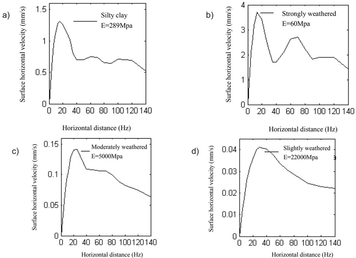
Fig. 9. The variation of surface horizontal velocity with horizontal distance.
