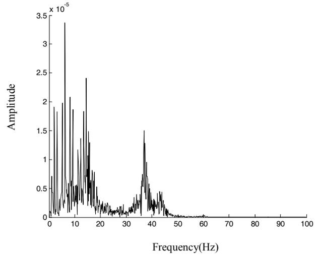
Fig. 22. Amplitude-frequency characteristic curve of vertical vibration velocity response at Sensitive Point 2.
