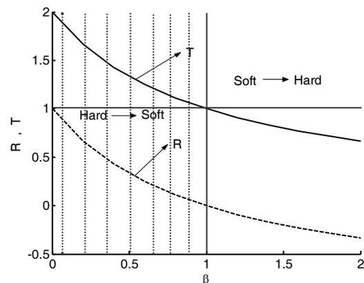
Fig. 6. The transmission coefficient and reflection coefficient of displacement wave.
