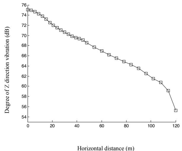
Fig. 27. Variation of Z vibration level with horizontal distance.
