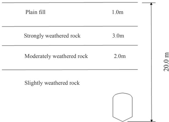
Fig. 16. The physical model of the stratum.
