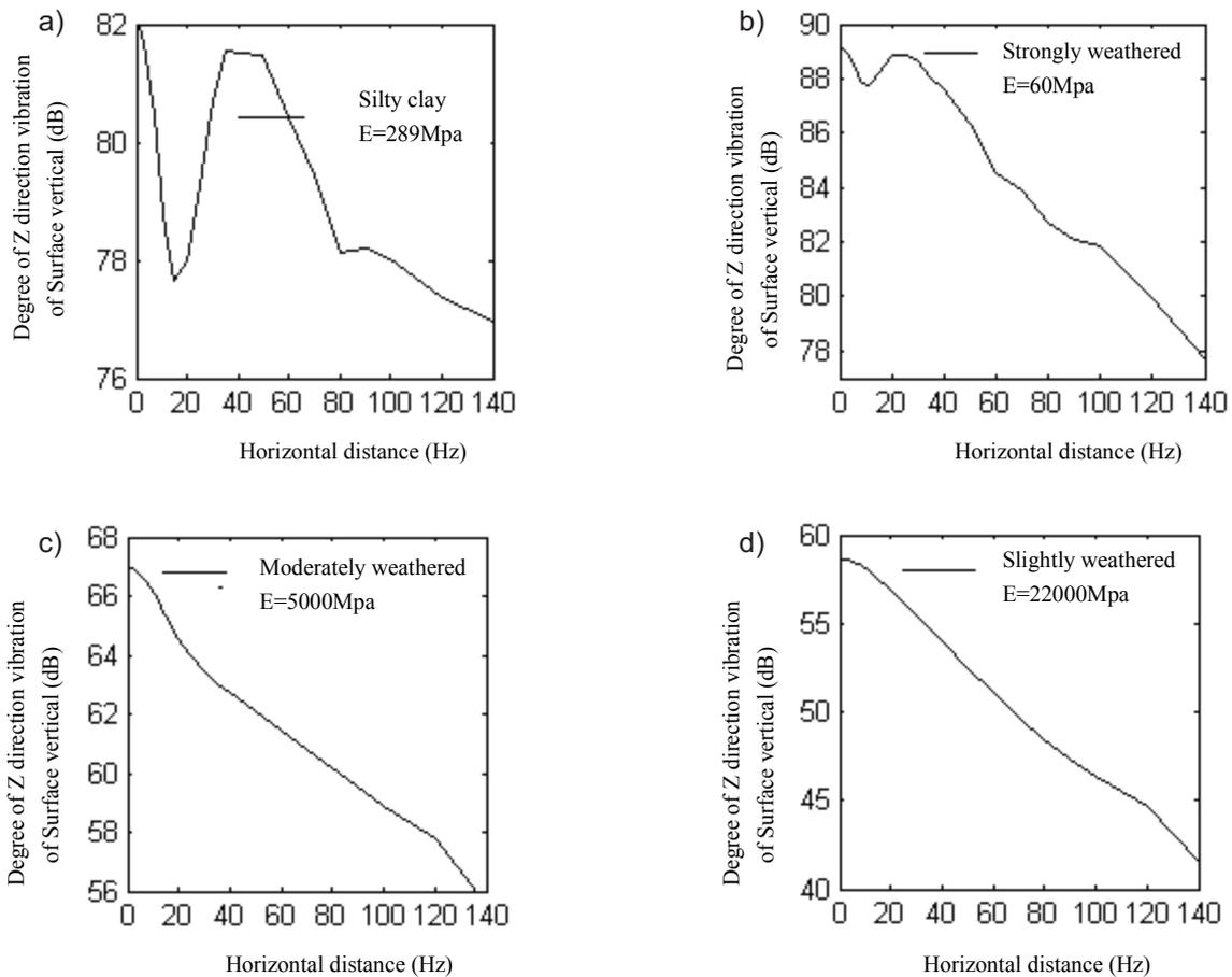
Fig. 10. The variation of degree of Z direction vibration of surface vertical with horizontal distance.
