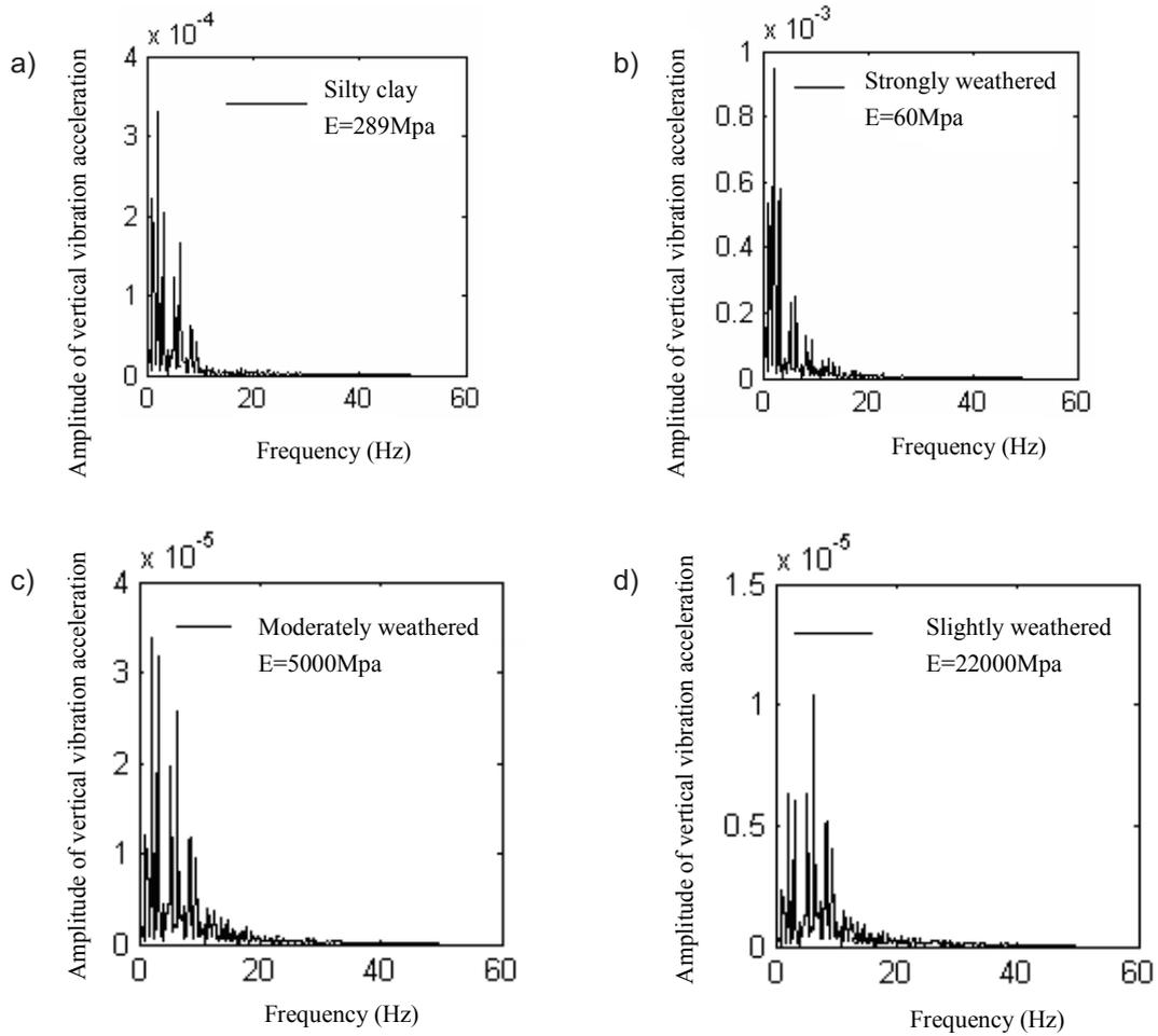
Fig. 8. Amplitude of vertical vibration acceleration at the center of the tunnel.
