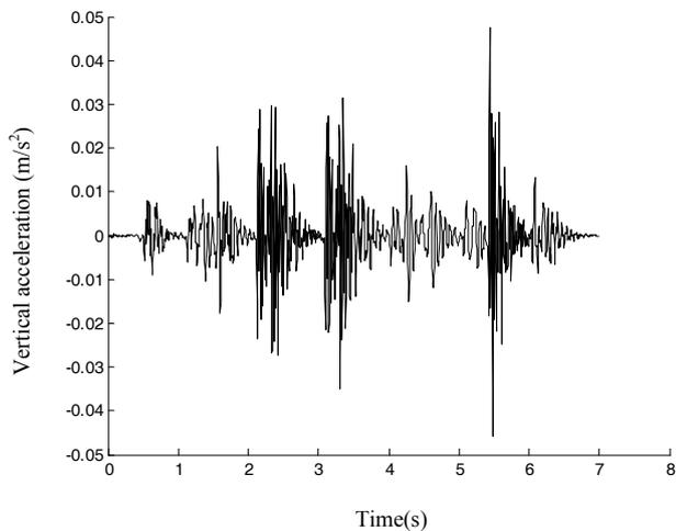
Fig. 21. Curve of vertical acceleration response with time at Sensitive Point 2.
