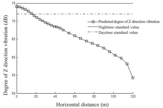
Fig. 28. The standard value of degree of Z direction vibration and its variation with horizontal distance.
