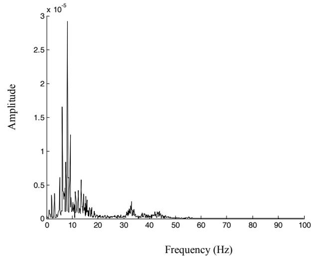
Fig. 18. Curve of horizontal velocity amplitude with frequency at Sensitive Point 1.
