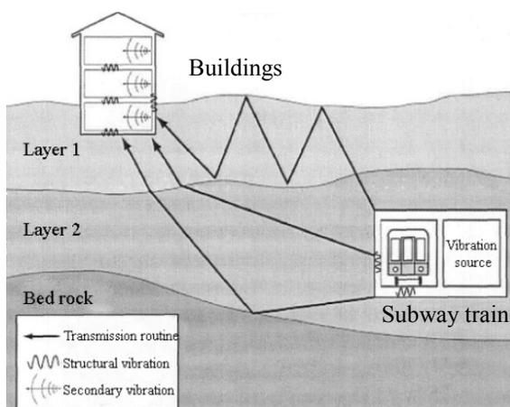
Fig. 1. The transmission of subway train vibration in rock stratum.
