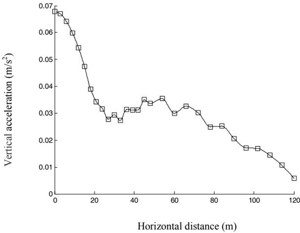
Fig. 25. Variation of vertical acceleration amplitude with horizontal distance.
