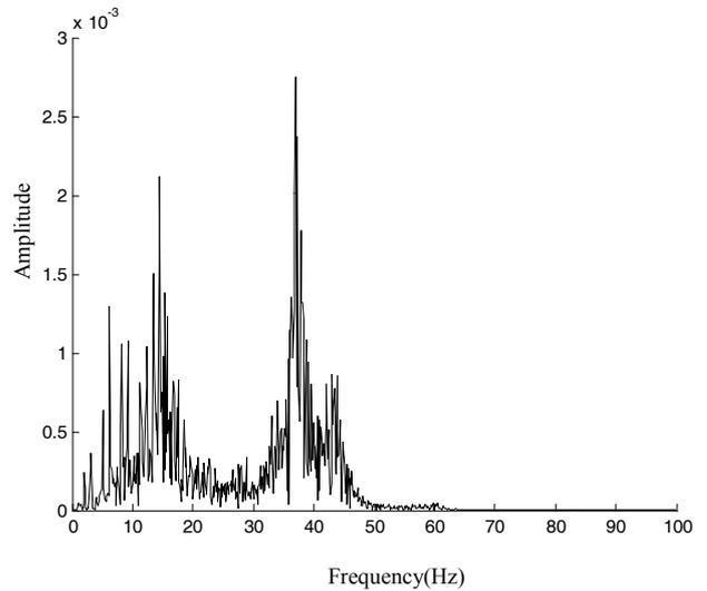
Fig. 23. Amplitude-frequency characteristic curve of vertical vibration acceleration response at sensitive point 2.
