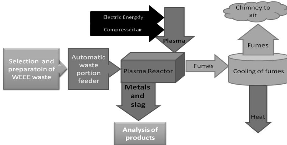
Fig. 2. Block diagram of the designed process for research on high-temperature plasma technology for metals recovery and waste neutralization.
