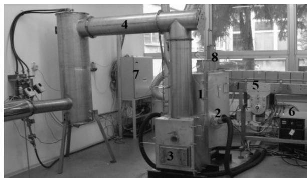
Fig. 1. Overview of the laboratory setup: 1) plasma reactor, 2) plasmatron, 3) molten product collection, 4) fume exhaust – chimney, 5) waste package transporter, 6) plasmatron power supply, 7) PLC – automation and data collection apparatus cabinet, 8) automatic waste package feeder.
