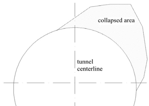
Fig. 2. Sketch map of the position of the collapse.
