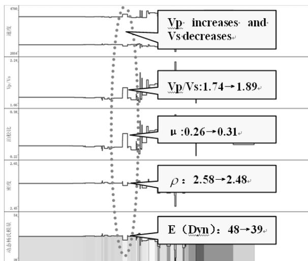
Fig. 5. Physical properties of the rock body.
