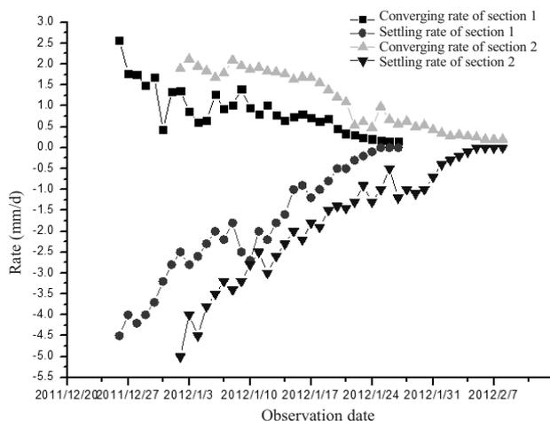
Fig. 9. Change curves of the convergence rate and crown settlement rate of the monitoring sections.
