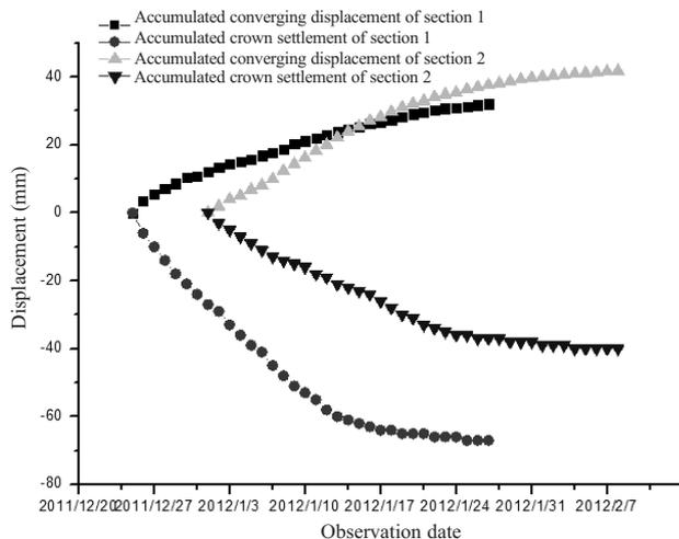
Fig. 8. Change curves of accumulated surrounding rock convergence and crown settlement of the monitoring sections.
