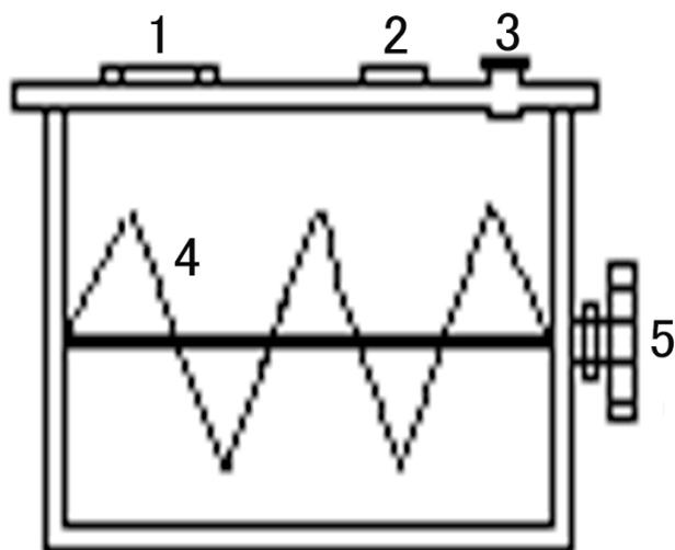
Fig. 1 Components of the experimental device (1 – feed opening, 2 – discharge opening, 3 – exhaust outlet, 4 – mixing mechanism, 5 – motor).
