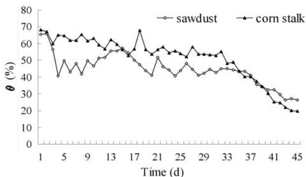
Fig. 3. Evolution of moisture content ( $\theta$ ) during the tests.
