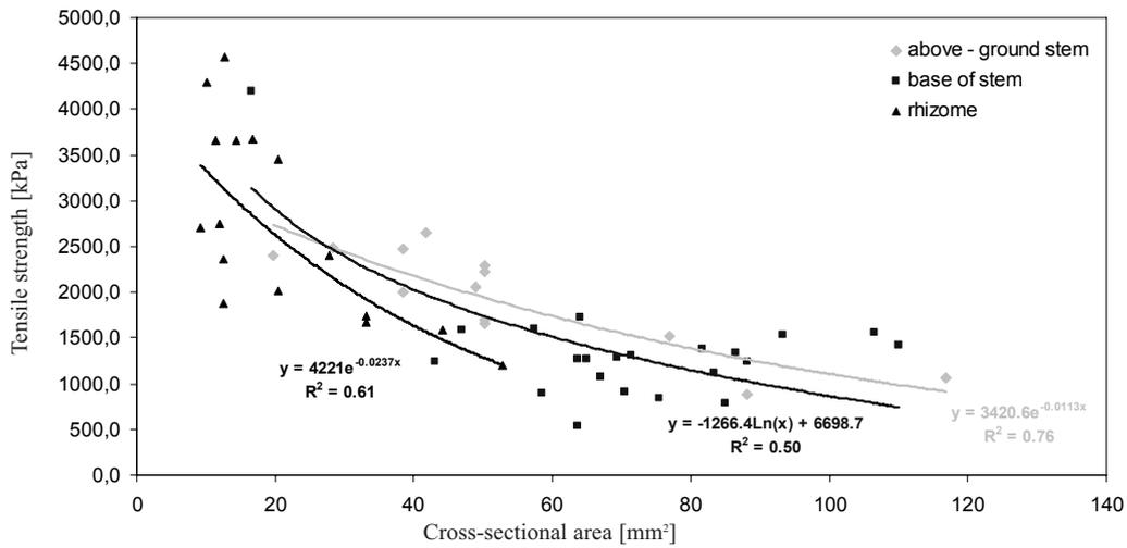
Fig. 4. Relationship between tensile strength and cross-sectional area of individual reed sweet grass parts.
