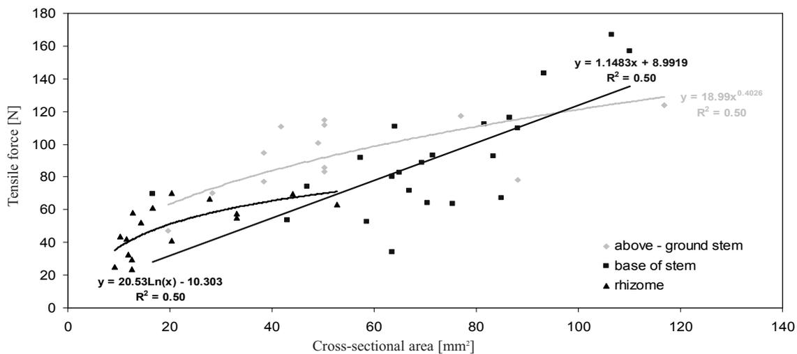
Fig. 2. Relationship between the tensile force and cross-sectional area of individual parts of reed sweet grass.
