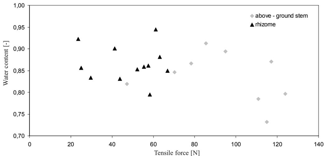
Fig. 3. Relationship between the water content and tensile force of individual parts of reed sweet grass
