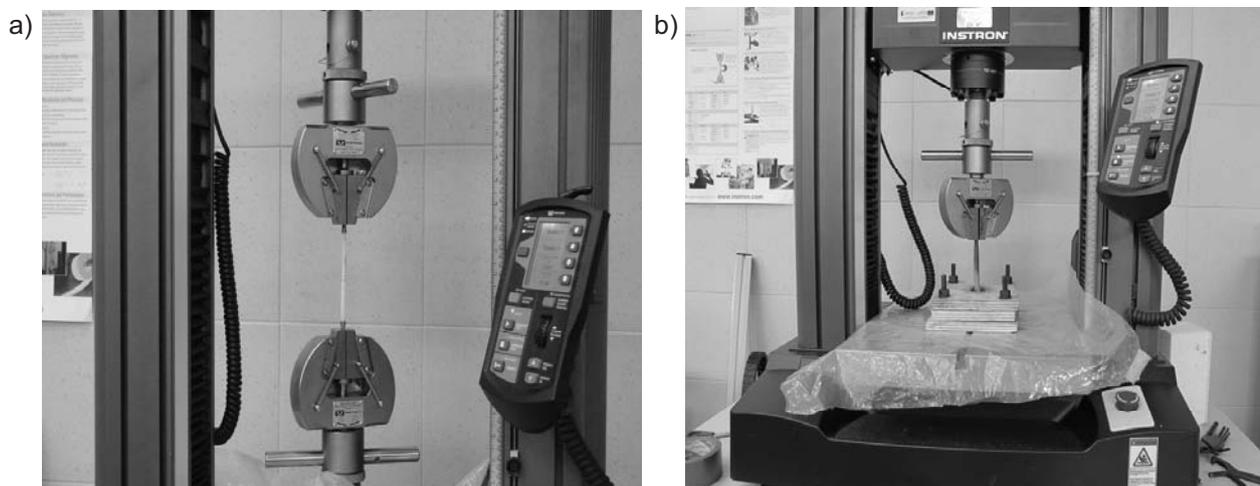
Fig. 1. Photographs illustrating clamps on an “Instron 5966” universal tensile strength testing machine used for measuring the tensile strength of the above-ground stem and rhizomes (a) and the base of the stem (b).
