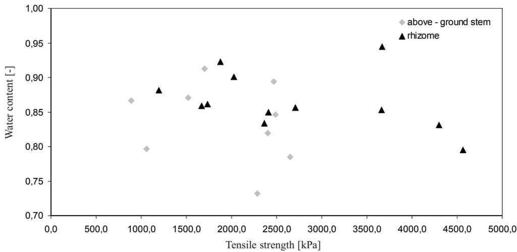
Fig. 5. Relationship between the water content and tensile strength of individual reed sweet grass parts.
